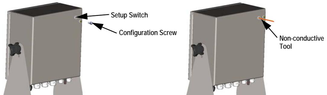
Figure 3-1. Setup Switch Location (Universal Enclosure)
