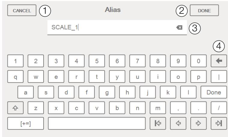
Figure 1-2. 1280 On-screen Full Keyboard for Alphanumeric Entry
