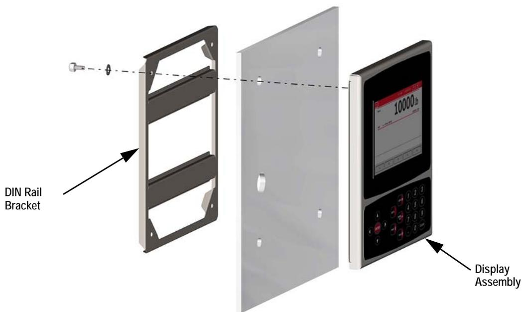
Figure 2-16. Mounting the 1280 - Panel Enclosure
