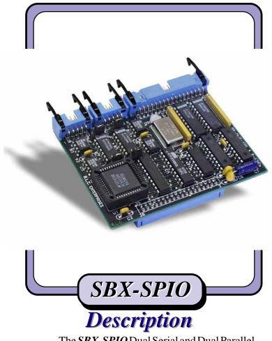
The *SBX-SPIO* Dual Serial and Dual Parallel I/O module provides two RS-232/422/485 ports and two 8-Bit Parallel Input/Output Ports. Both serial ports provide full duplex serial communication with hand-shaking lines. Both serial ports provide high speed interrupt driven sixteen byte FIFO's (16C552) for both receive and transmit data. RS-422 and multi-drop RS-485 drivers with tri-state transmitter control is also provided.
