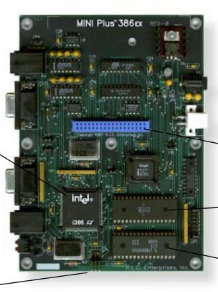
Battery Back-Up Real Time Clock Static RAM
