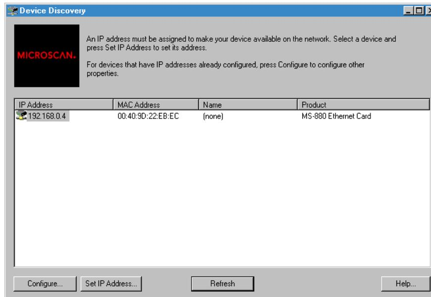
3. If the hardware is installed properly and DHCP is part of your network, the IP and MAC address will appear on the screen above.
