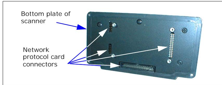
Figure 1-1 Bottom of MS-880 Scanner
