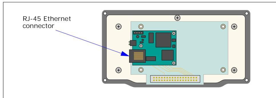
Figure 4-2 Bottom Plate with Ethernet Card Attached
