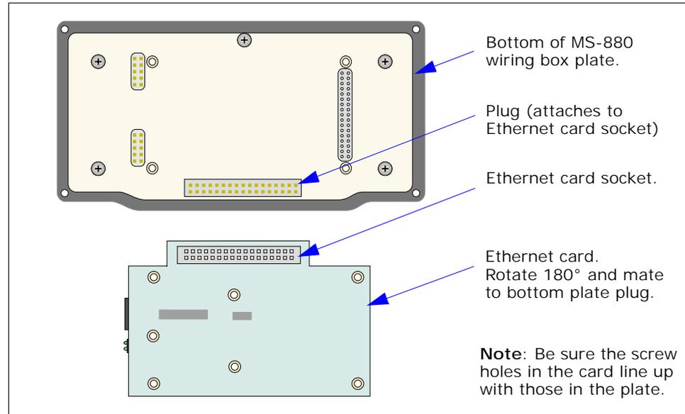
Figure 4-1 Bottom Plate and Ethernet Card (unassembled)
