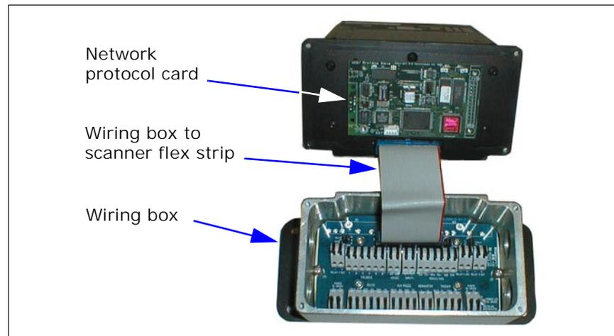
Figure 1-1 MS-880 Scanner, Wiring Box and Network Card
