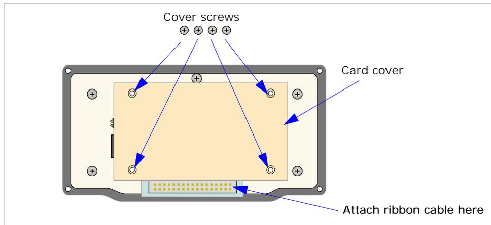
Figure 4-3 Ethernet Card (with cover)
