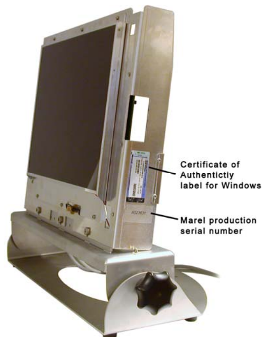
Figure 13 M6000 Controller, location of the Certificate of Authenticity label for Windows.
