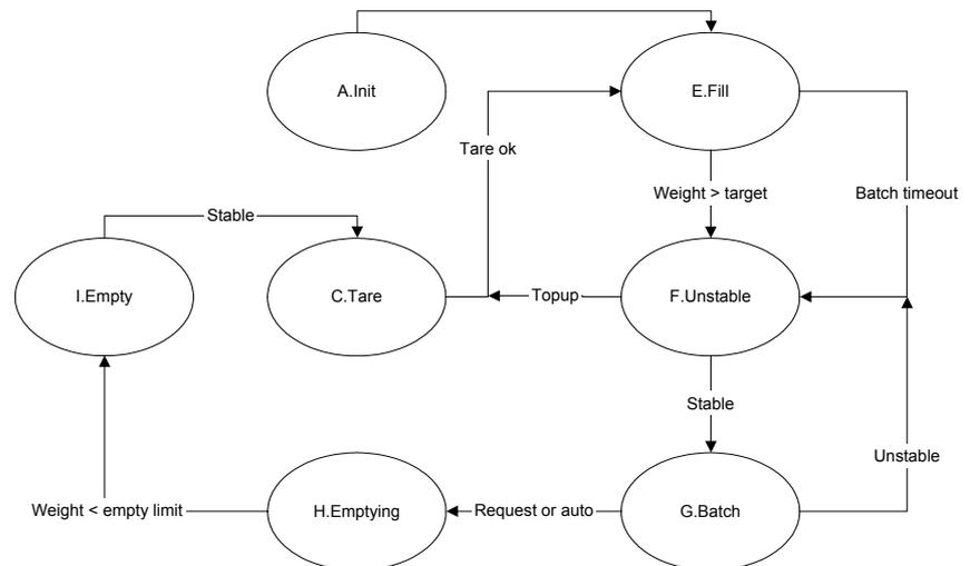
Figure 7 Weighing cycle with state labels.
