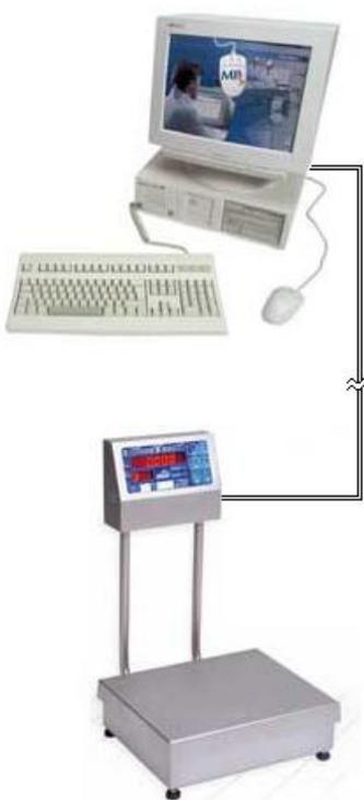
The M1100 can communicate with external equipment using the RS-232 port. Weighing results can be printed on an external printer or the data can be transmitted to a PC for storing and further processing. The M1100 settings can also be changed by transmitting serial commands from a PC.
