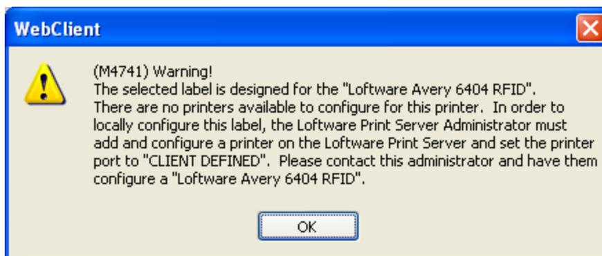
Figure 9.10: Request for CLIENT DEFINED Printer for Label
