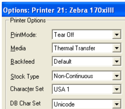
Figure 7.2: Character Set settings in Printer Options (Per-printer)
