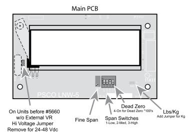
The Lift-N-Weigh is normally pre-calibrated to the customer supplied lift truck specifications. This is a test bench calibration to the calculated pressure. Because of friction in the lifting mechanism and control valve bleedback, weight errors may exist in the system when installed on the customers equipment. These can often be easily corrected by performing the following adjustments:
