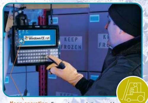
**Keep operating.** Frequent moves between cold and ambient temperatures won't disrupt this operator's productivity. Heaters, coatings and sealing protect from condensation.
