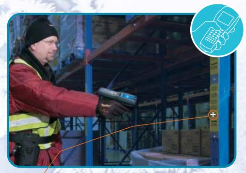
**Keep scanning.** Bar codes can be read efficiently since the built-in heater prevents the scan window from fogging up.
