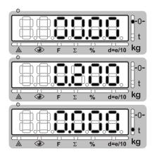
5.2.2 <u>LEFT ARROW KEY</u>: This is used to move the selected digit while entering settable values or calibration weight or any other user parameter etc.
