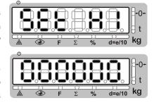
sound will be there that is you have to lift the excess weight from the pan. The high low limit enunciator shows the status of weight range is either HI / LO / OK
