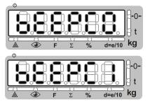
completmented to sound above 100g and remain disabled when the reading is below100g. The alarm does not sound at 0 level or 0 level + 3 divisions.
