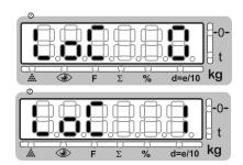
inactive and LOC 1 means setting is active and keyboard is locked.
