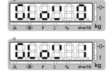
When the indicator is in the weighing mode, While pressing the ZERO button, press the TARE button. The display will show "P-TARE" Now press the ENTER button two times so that the display shows "GLOW O". O means the GLOW
