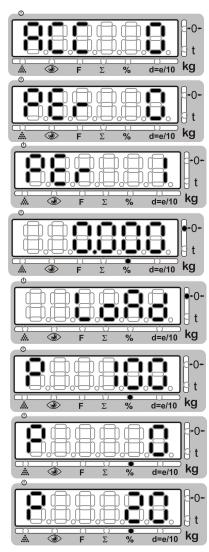
that is 30% of the sample weight. Also the RED LED corresponding to P on the panel sticker will alow, indicating that the indicator is in the percentage
