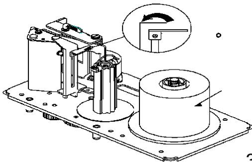
3. Peel-off and discard about 3 labels and install paper roll.
