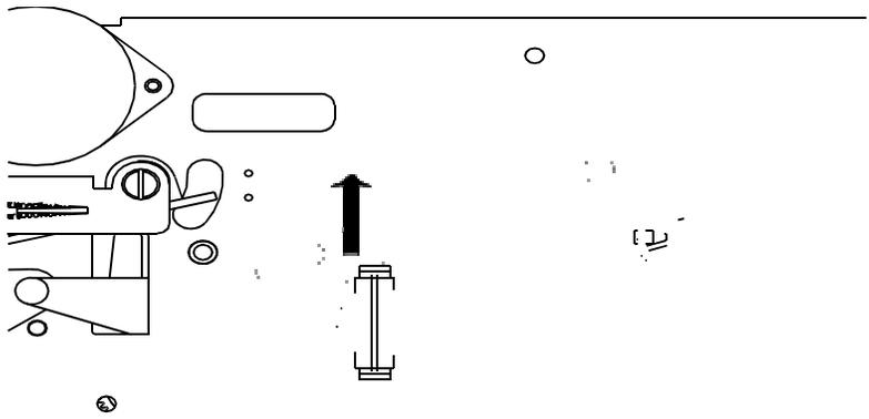
4. Pull out paper retaining spring. Feed the backing paper around the pickup spool.
