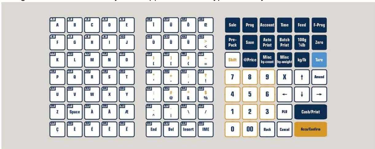
There are 63 speed keys placed in the first two panels starting from the left. Each speed key has its address printed on the top left corner.
