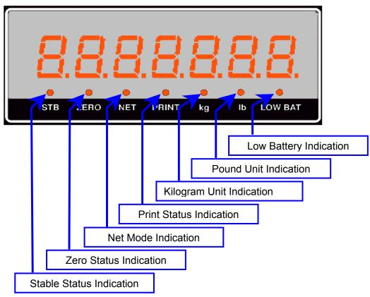
There are 7 LED indicators just below the 7-segment weight display with the following functions.
