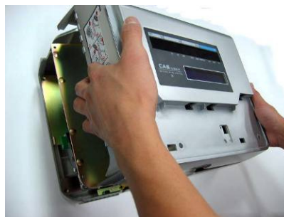
Open up from printer side to disassemble front cover
