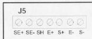
Figure 2-6: Connection assignments for the Load Cell Terminal (J5)
