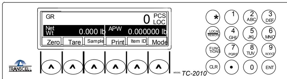
FIGURE 1-1: TC-2010 Series Front Panel
