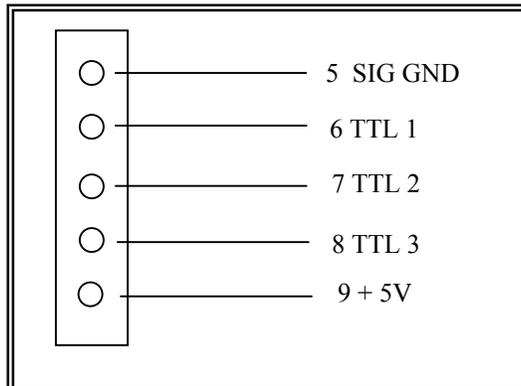
**FIGURE B-2: Cable Diagram for Scale to external relays**
