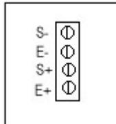
*Figure 2-2: Connection assignments for the Load Cell Terminal*
