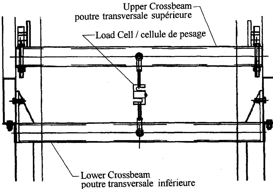
**LOAD CELL MOUNTING / Montage de la cellule de pesage****EVALUATED BY:**
