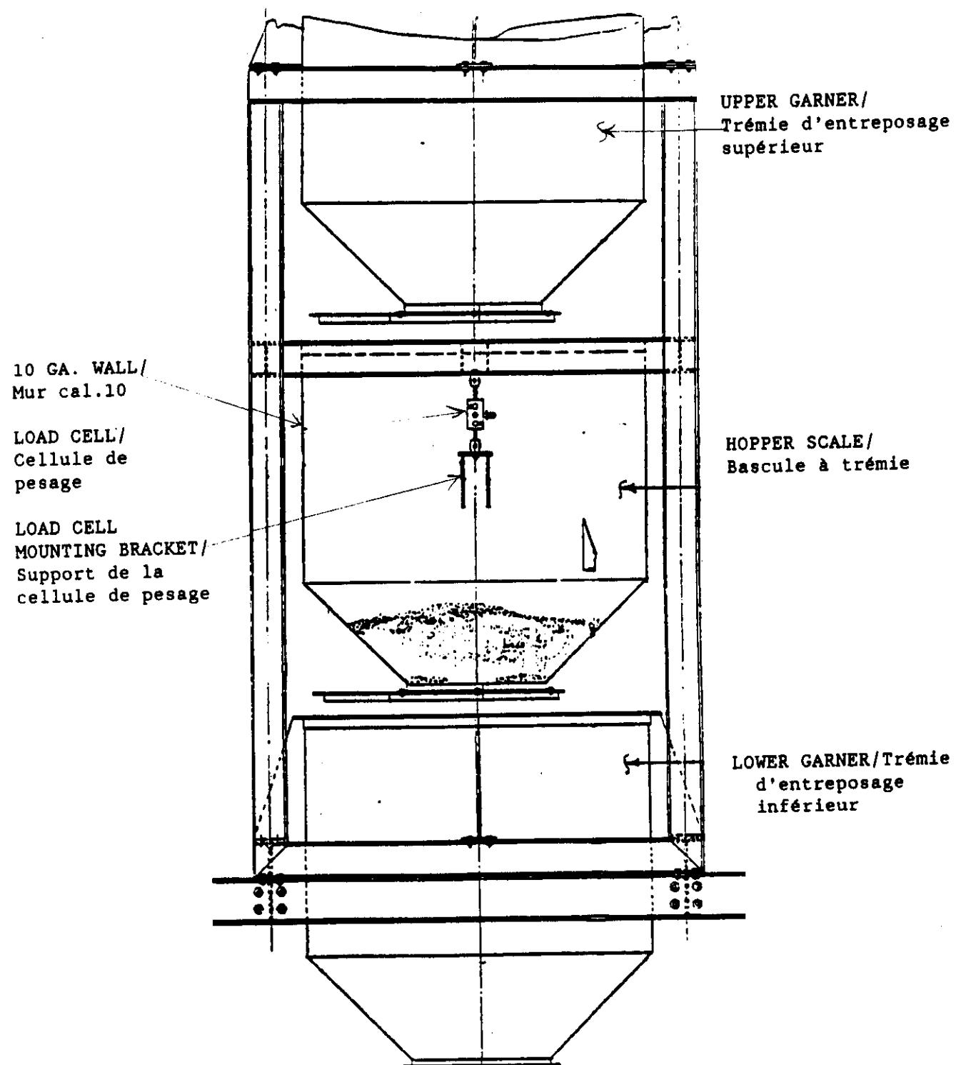
TYPICAL BULK WEIGHING SYSTEM
