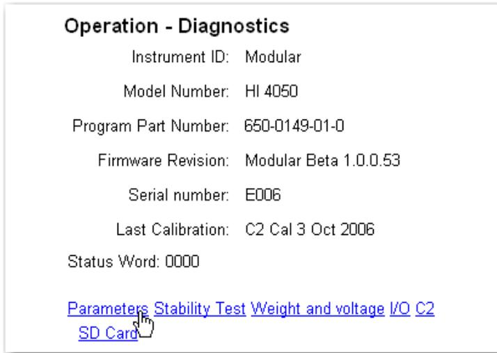
**FIG. 354 DIAGNOSTICS PAGE/SELECTING PARAMETERS**
