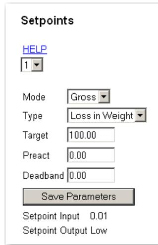
The screenshot shows the same "Setpoints" window. The "Type" dropdown is now closed and set to "Loss in Weight". The "Target" field is now highlighted with a blue selection bar and contains the value "100.00". All other fields and the "Save Parameters" button remain the same as in the previous figure.
