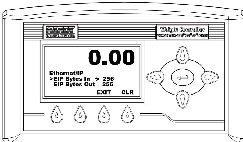
**FIG. 130 ETHERNET/IP MENU/SELECTING EIP BYTES IN**
