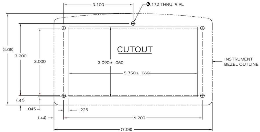
**FIG. 3 PANEL HOLE DIMENSIONS (RETROFIT)**
