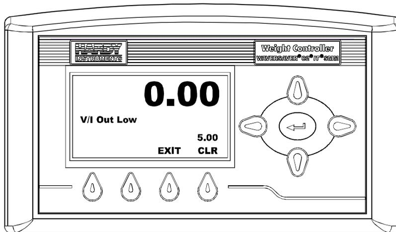
**FIG. 150 ADJUSTING V/I OUT LOW TO 5.0 VOLTS**
