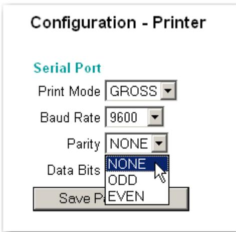
**FIG. 205 PRINTER SETUP/SELECTING PARITY**
