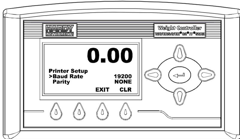
**FIG. 92 PRINTER SETUP MENU/SELECTING BAUD RATE**
