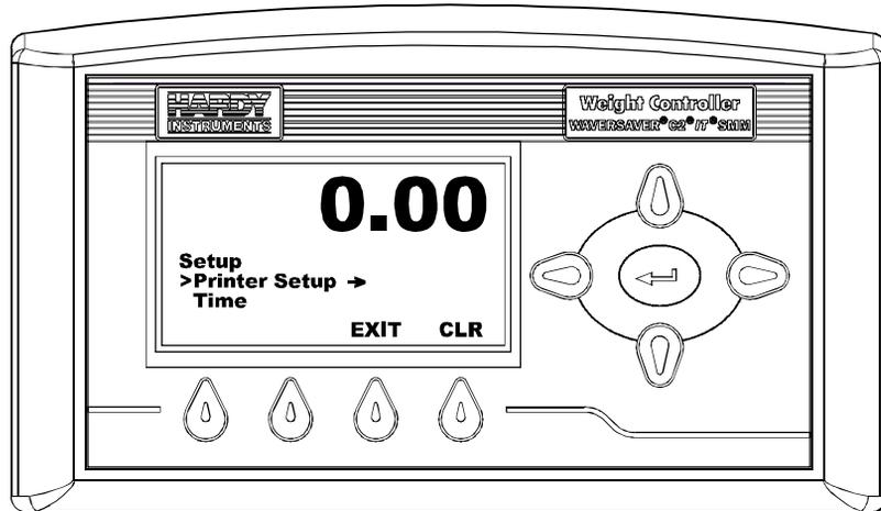
**FIG. 90 SETUP MENU/SELECTING PRINTER SETUP**
