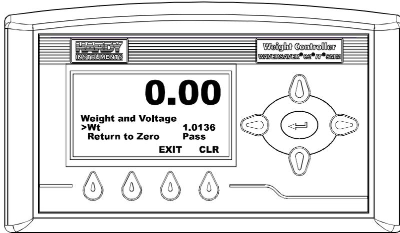
**FIG. 400 WEIGHT AND VOLTAGE TEST/WEIGHT AND RETURN TO ZERO RESULTS**
