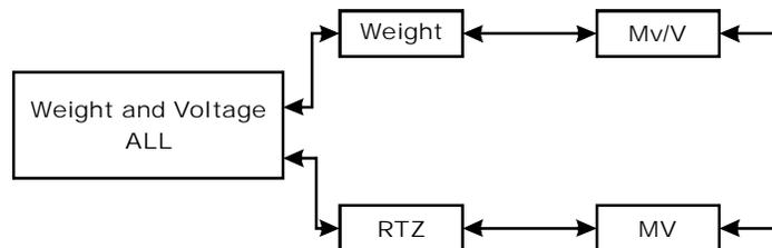
This test section looks at the readings from ALL the load cells. This test works for all varieties of load cell connection systems. This will test overall system performance and signal voltage readings. Further investigation to isolate system problems require the use of hand tools and multi-meters or the Integrated Technician Summing Junction Box and using the IT<sup>®</sup> Test section.
