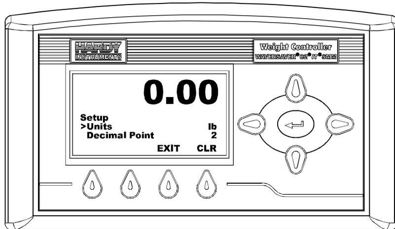
**FIG. 67 CONFIGURATION/SETUP MENU/SELECTING UNITS OF MEASURE**
