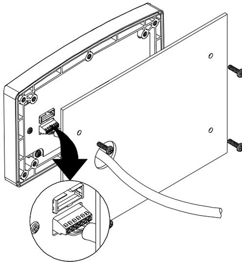
**FIG. 13 REMOTE DISPLAY ONLY CONNECTING TO DISPLAY BOARD**
