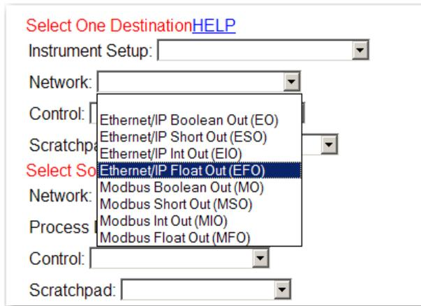
**FIG. 330 NETWORK/SELECTING ETHERNET/IP FLOAT OUT (EFO)**
