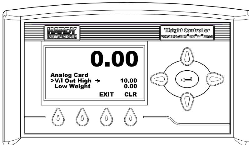
**FIG. 151 ANALOG CARD MENU/SELECTING V/I OUT HIGH**
