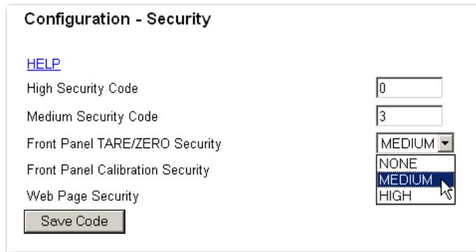
The screenshot shows the same "Configuration - Security" window. In addition to the two text input fields, there are two pull-down menus. The first is labeled "Front Panel TARE/ZERO Security" and is currently set to "MEDIUM". The second is labeled "Front Panel Calibration Security" and is currently set to "MEDIUM". A mouse cursor is pointing at the "MEDIUM" option in the second pull-down menu. At the bottom left of the window is a "Save Code" button.
