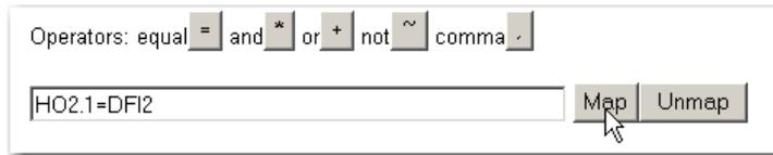
**FIG. 349 ASSIGNMENT STATEMENT MAPPING DEVICENET FLOAT IN (DFI2) TO ZERO (HO2.1)**
