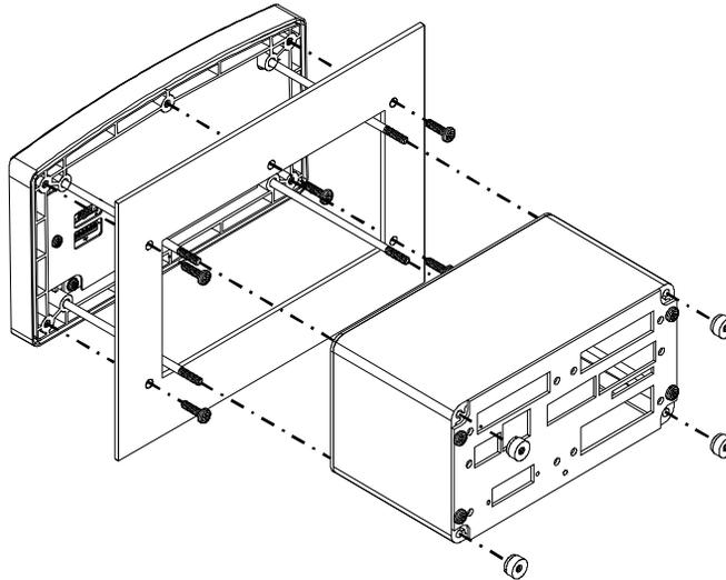
**FIG. 6 RETROFIT PANEL MOUNT INSTALL FOR HI 2151/30 & HI 2110**
