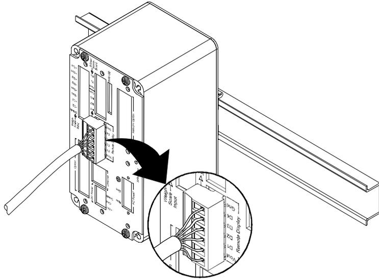
**FIG. 11 CONNECTING DISPLAY CABLE TO ELECTRONIC ENCLOSURE**
