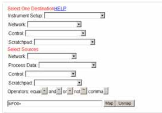
**FIG. 237 MAPPING DISPLAY/SELECTING DESTINATION: MFO0 (MODBUS FLOAT OUT - WORD 0)**
