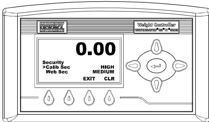
**FIG. 289 SECURITY MENU/SETTING PASSWORDS FOR CALIB AND WEB SECTIONS**
