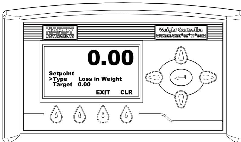
**FIG. 366 SET POINT MENU/SELECTING LOSS IN WEIGHT**
