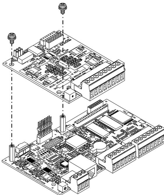
**FIG. 25 ALIGNING THE ANALOG OUTPUT CARD WITH THE BOARD STACKER PINS AND STANDOFFS**
