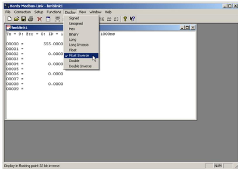
**FIG. 242 HARDY MODBUS-LINK DISPLAY/SELECTING DISPLAY/FLOAT INVERSE**
