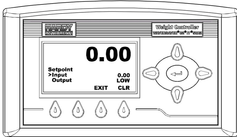
**FIG. 64 SETPOINT MENU/READING INPUT**
