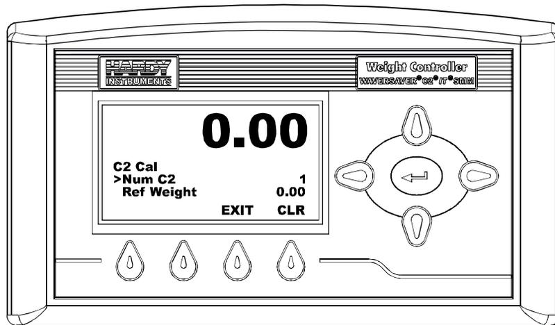
**FIG. 306 C2 CALIBRATION MENU/SELECTING NUMBER OF C2 LOAD CELLS**
