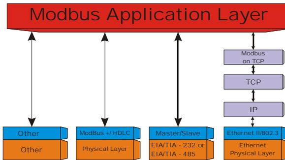
**FIG. 223 MODBUS COMMUNICATION DIAGRAM**
