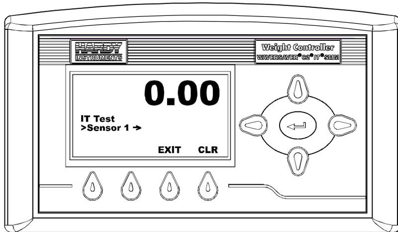
**FIG. 403 IT TEST/SELECT SENSOR 1**
