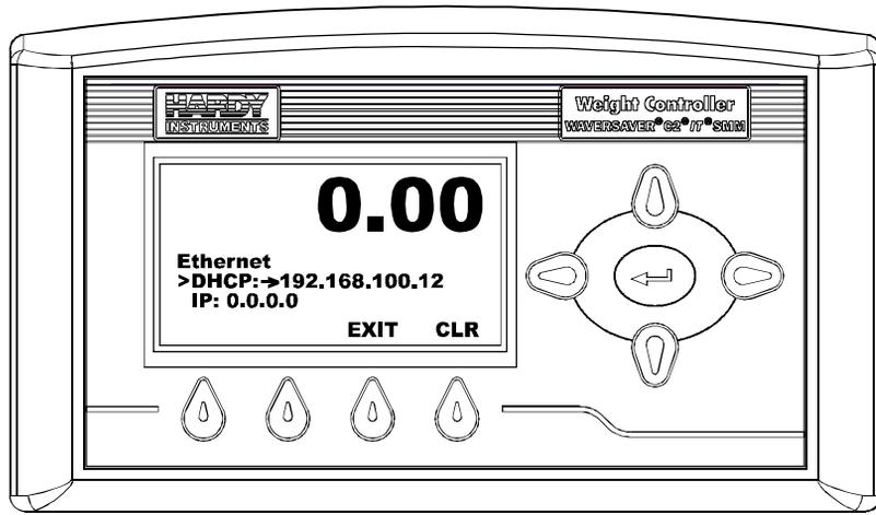
**FIG. 113 ETHERNET MENU/DHCP DOES NOT SHOW ALL THE IP ADDRESS**
