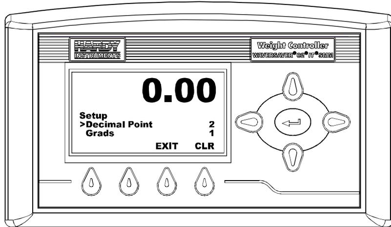
**FIG. 69 SETUP MENU/SELECTING DECIMAL POINT POSITION**
