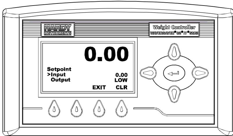
**FIG. 373 SETPOINT MENU/READING INPUT**
