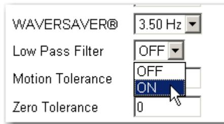
**FIG. 196 INSTRUMENT SETUP/LOW PASS FILTER**
