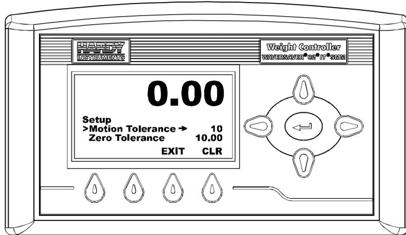
**FIG. 75 SETUP MENU/SELECTING MOTION TOLERANCE**
