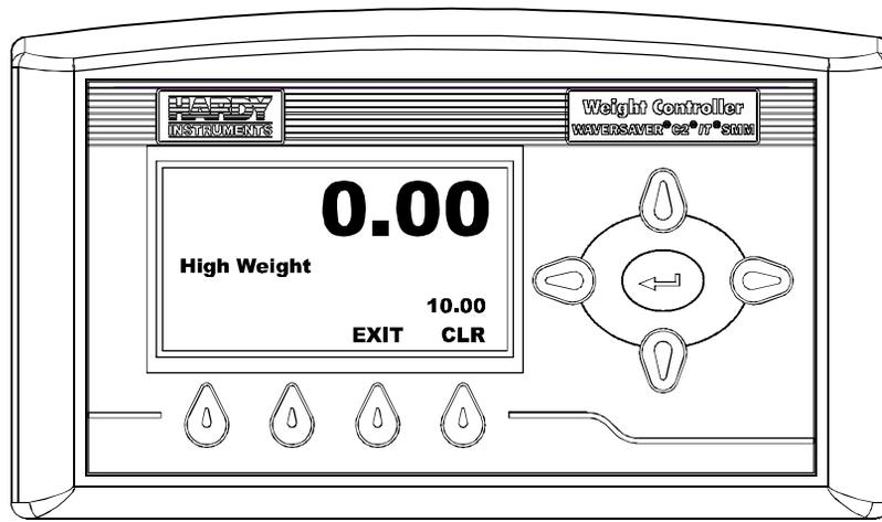
**FIG. 156 HIGH WEIGHT MENU/SETTING HIGH WEIGHT**
