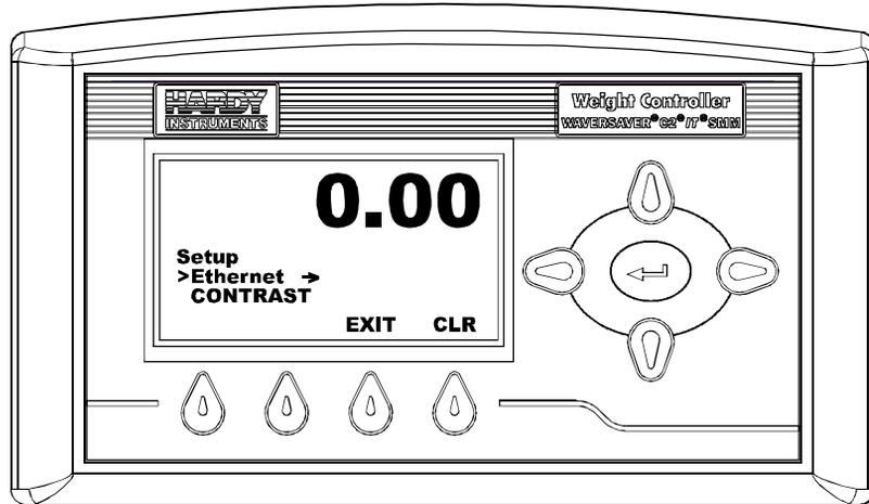
**FIG. 108 SETUP MENU/SELECTING ETHERNET**
