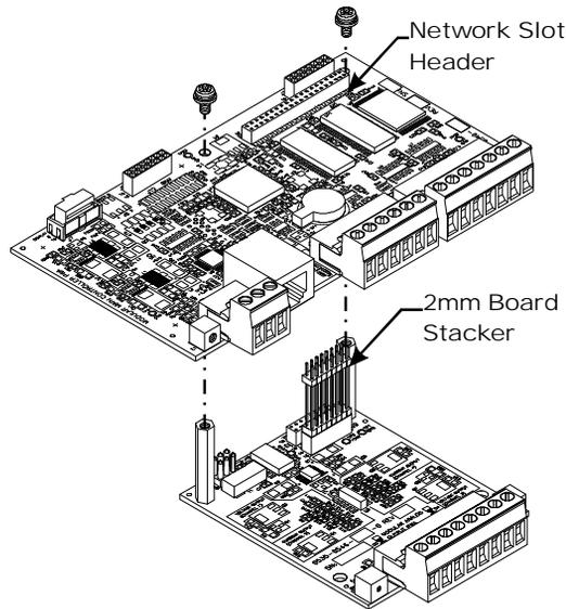
**FIG. 21 ALIGNING THE BOARD STACKER PINS WITH THE NETWORK HEADER HOLES IN THE MAIN CONTROL BOARD**
