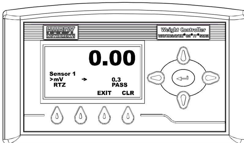
**FIG. 405 SENSOR 1 MENU/SETTING MILLIVOLTS**
