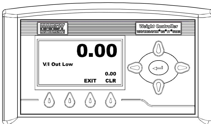
**FIG. 149 V/I OUT LOW MENU/SETTING LOW OUTPUT VOLTAGE**
