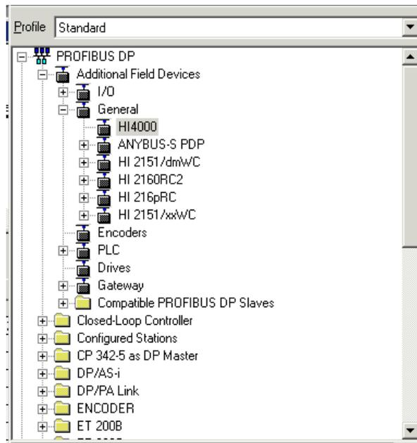
**FIG. 162 HARDWARE CATALOG/SELECTING HI 4000 PDP FOLDER**
