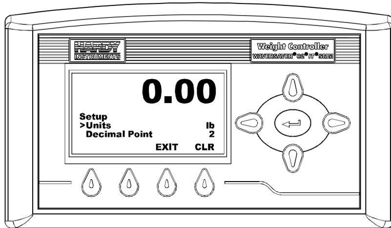
**FIG. 68 SETUP MENU/SELECTING UNITS**
