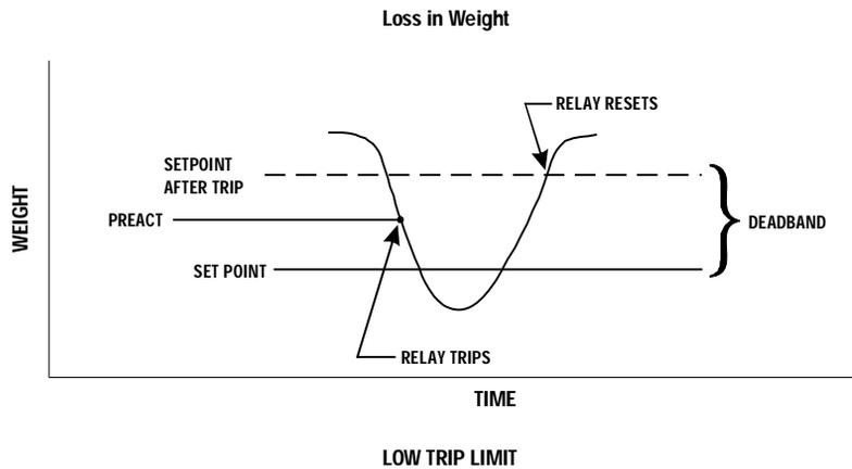
**FIG. 376 LOSS IN WEIGHT/LOW TRIP LIMIT**
