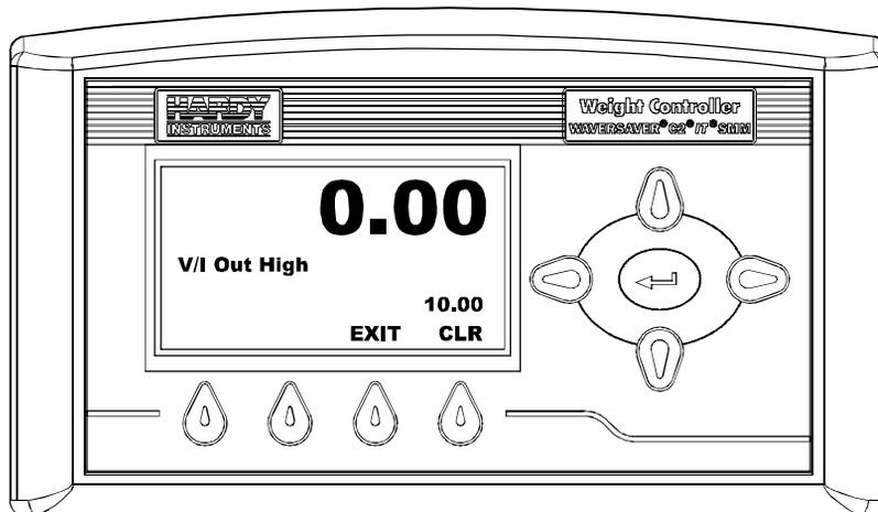
**FIG. 152 V/I OUT HIGH MENU/SETTING HIGH VOLTAGE**
