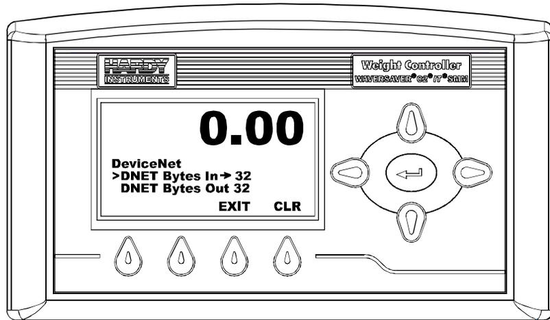
**FIG. 121 DEVICENET MENU/SELECTING DNET BYTES IN**
