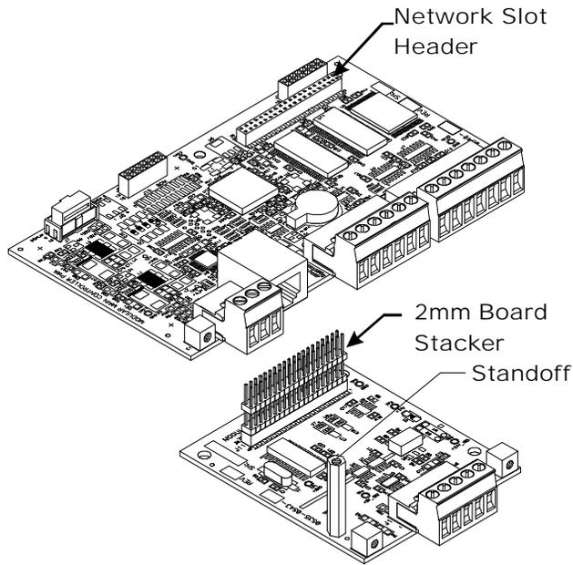
**FIG. 35 INSTALLING DEVICENET CARD**
