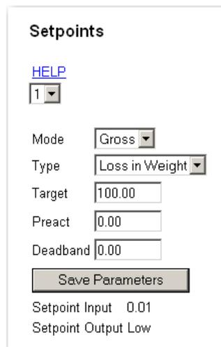
The screenshot shows the same "Setpoints" window. The "Type" dropdown is now closed and set to "Loss in Weight". The "Target" text field is highlighted with a blue selection bar and contains the value "100.00". The "Preact" text field contains "0.00". The "Deadband" text field contains "0.00". The "Save Parameters" button is visible. At the bottom, it displays "Setpoint Input 0.01" and "Setpoint Output Low".
