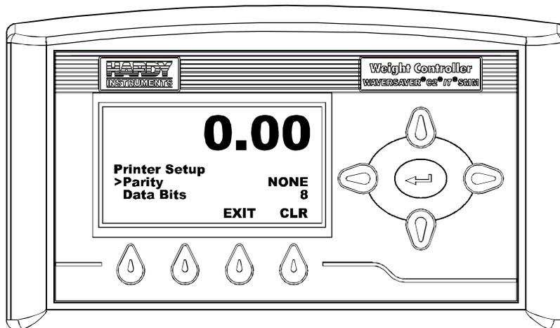
**FIG. 93 PRINTER SETUP MENU/SELECTING PARITY**
