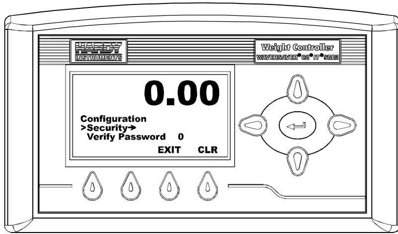
**FIG. 277 CONFIGURATION MENU/SELECTING SECURITY**
