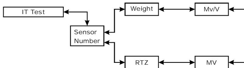
If your system is equipped with an Integrated Technician Summing Junction box the IT test can help identify individual load cell problems up to a maximum of four load cell selections.
