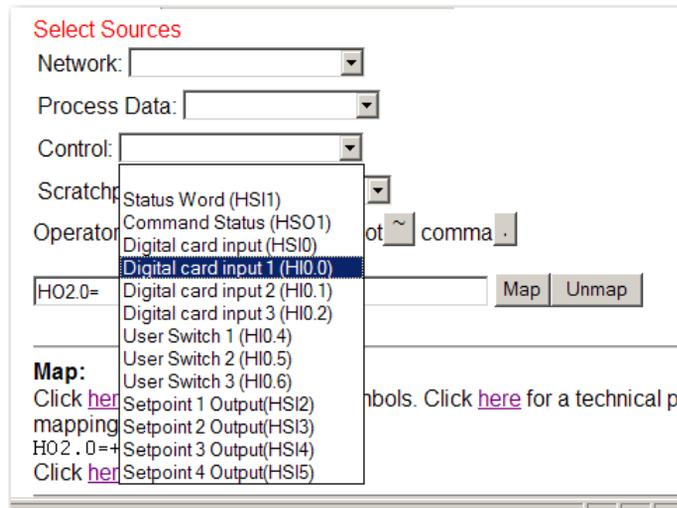
**FIG. 267 SOURCES/SELECTING DIGITAL CARD INPUT 1**
