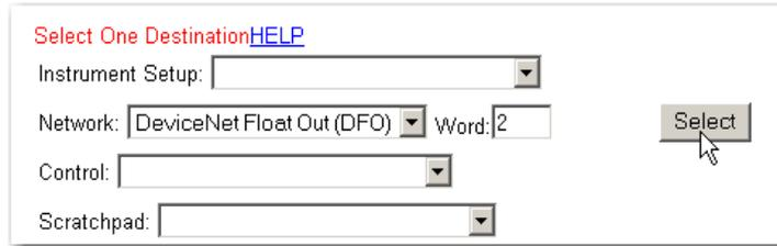
The screenshot shows a dialog box titled "Select One Destination" with a "HELP" link. It contains four dropdown menus: "Instrument Setup", "Network" (set to "DeviceNet Float Out (DFO)"), "Control", and "Scratchpad". To the right of the "Network" dropdown is a text box labeled "Word:" containing the number "2". A "Select" button is located to the right of the "Word:" text box, with a mouse cursor pointing at it.
