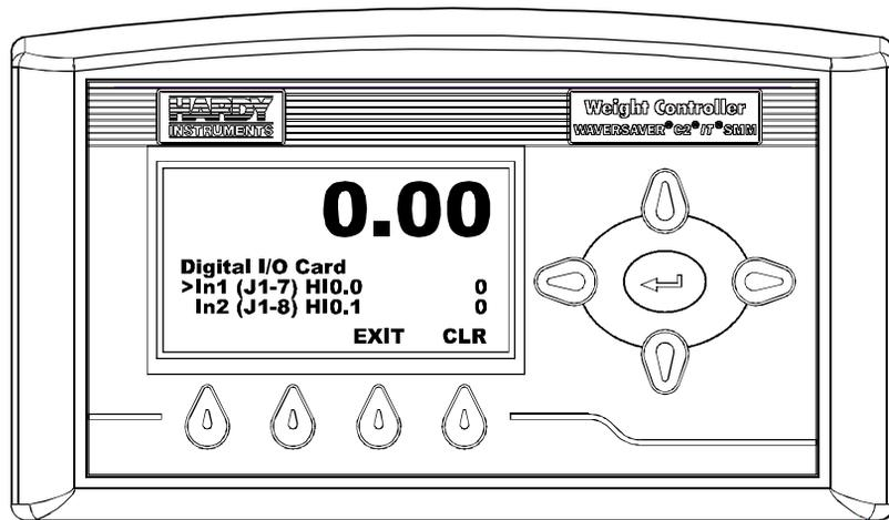
**FIG. 160 DIGITAL I/O CARD/READING INPUT 1**
