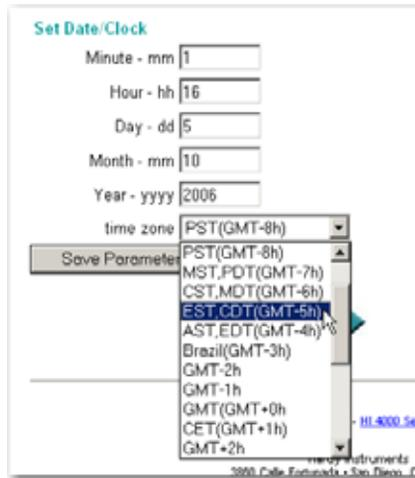
**FIG. 213 DATE/TIME SETUP/SELECTING GREENWICH TIME**
