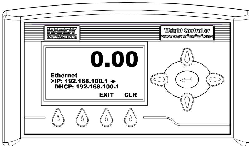
**FIG. 109 ETHERNET MENU/SELECTING IP**
