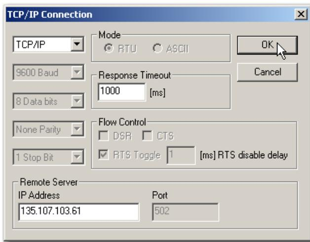
**FIG. 232 TCP/IP CONNECTION DISPLAY/ENTERING THE IP ADDRESS**
