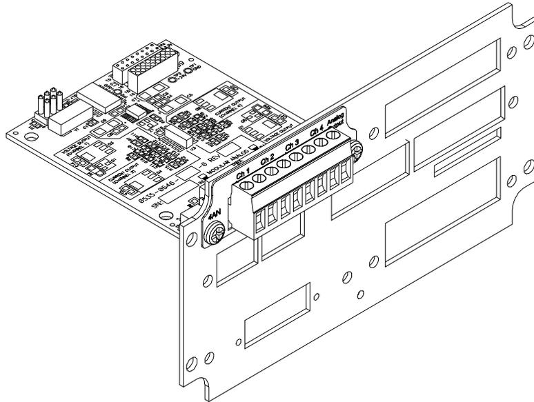
**FIG. 27 ANALOG CARD (-4ANB) CONNECTED TO REAR PANEL**
