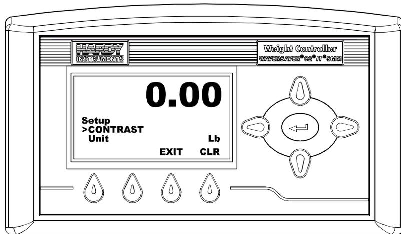
**FIG. 115 SETUP MENU/SELECTING CONTRAST**
