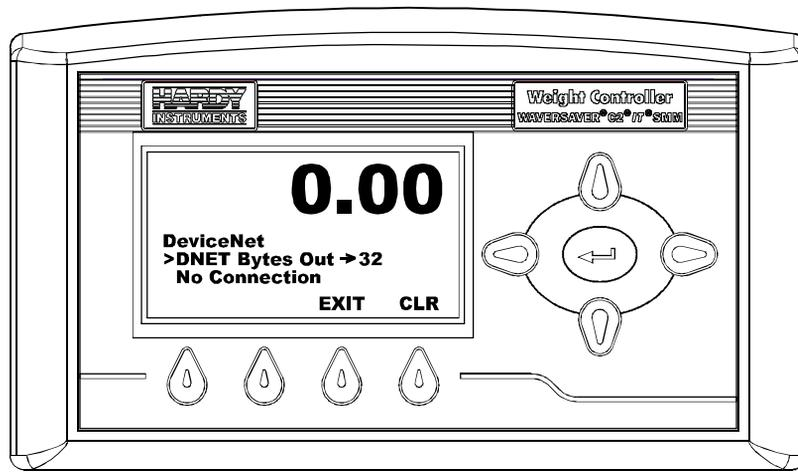
**FIG. 125 DEVICENET MENU/NO CONNECTION**
