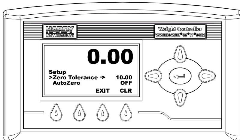
**FIG. 77 SETUP MENU/SELECTING ZERO TOLERANCE**
