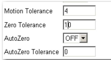
A screenshot of a configuration dialog box with four rows. The first row is 'Motion Tolerance' with a text field containing '4'. The second row is 'Zero Tolerance' with a text field containing '10'. The third row is 'AutoZero' with a dropdown menu set to 'OFF'. The fourth row is 'AutoZero Tolerance' with a text field containing '0'.
