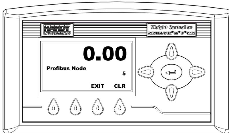
**FIG. 173 PROFIBUS NODE MENU/SELECTING NODE ADDRESS NUMBER**
