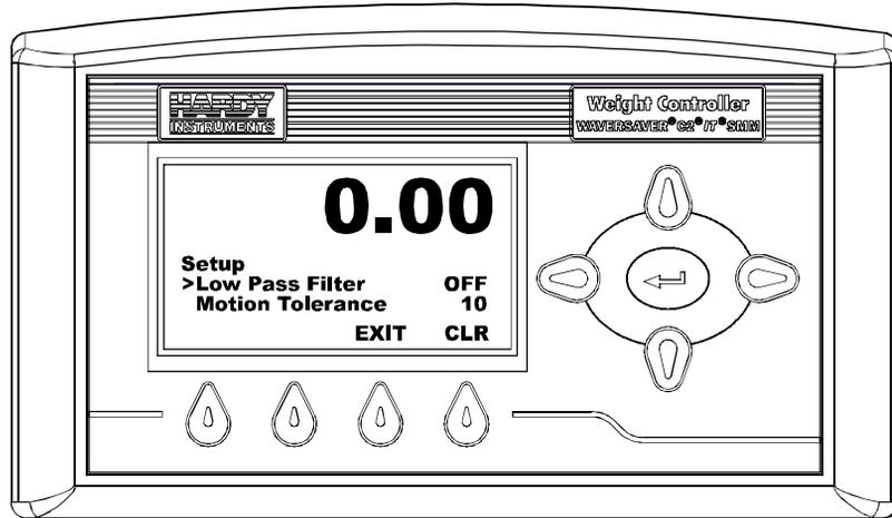
**FIG. 74 SETUP MENU/SETTING LOW PASS FILTER**
