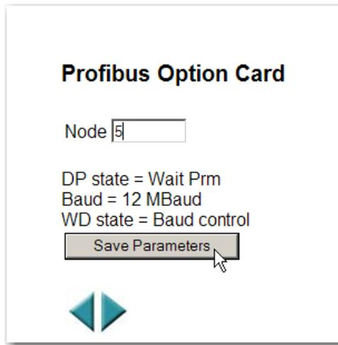
**FIG. 276 PROFIBUS OPTION CARD/ENTERING NODE ADDRESS**
