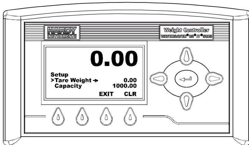
**FIG. 82 SETUP MENU/SELECTING TARE WEIGHT**
