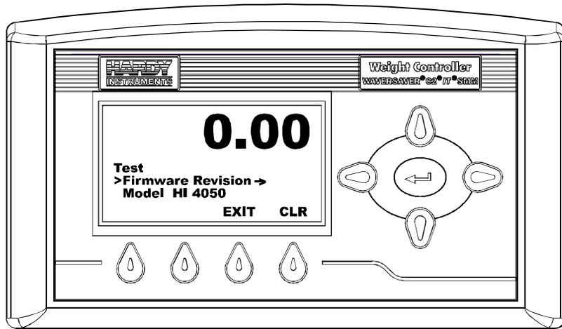
**FIG. 389 TEST MENU/SELECTING FIRMWARE REVISION NUMBER**
