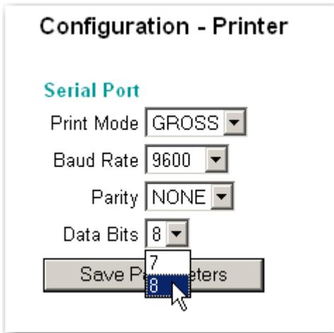
**FIG. 206 PRINTER SETUP/SELECTING DATA BITS**
