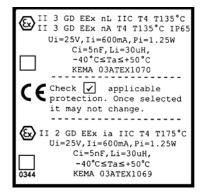
If you install a load cell in a hazardous area, use a permanent marker to place a mark in the check box on the label that indicates the applicable protection (KEMA 03ATEX1069 or KEMA 03ATEX1070). Once the label has been marked, it may not be changed.
