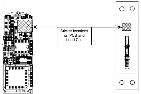
Un-matched load cells and PCBs may not perform correctly in a scale unit. The part numbers for a load cell and pcb pair are listed below:
