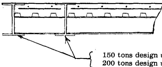
150 tons design uses 8"x21" main I beams
