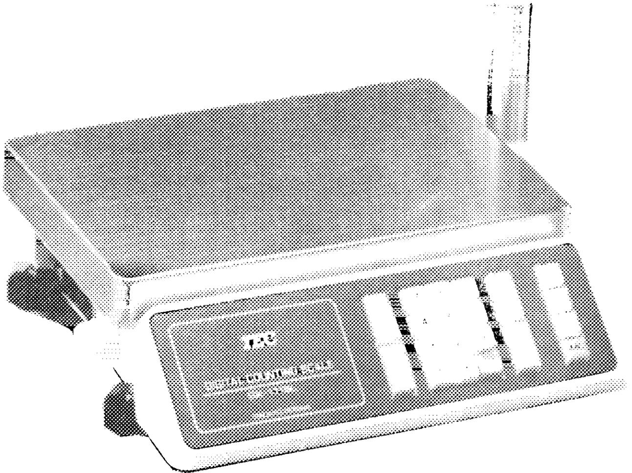
Description: These devices are electronic load cell scales with counting features composed of a weighing element and a weight indicator. These scales are micro-processor controlled and utilize a cantilever type load cell. The micro-processor system is used to compute weight in lb and kg. The indicator has one display panel for the operator to indicate modes of operations i.e.; weight, tare, zero, weight/piece in lbs. or kg. and count. The operator controls located on the front of the scale are:
