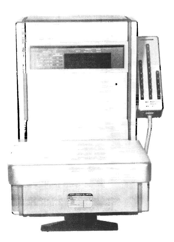
The base and other structural members are of die-cast alloy. The enclosure is of polished sheet aluminum.
