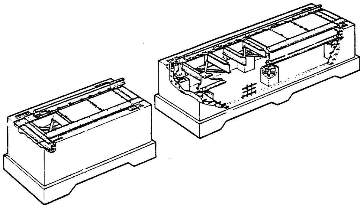
Description: This device is a railroad track scale utilizing Toledo cannister load cells with a cap-check and rocker pin mechanism providing a self-contained suspension system.
