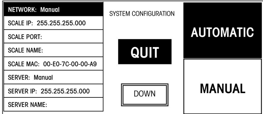
**Figure 3-1: Network Setup Menu Screen One**
