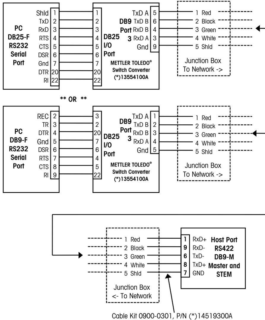
SmartTouch® Master or STEM RS422 to METTLER TOLEDO® Converter Wiring
