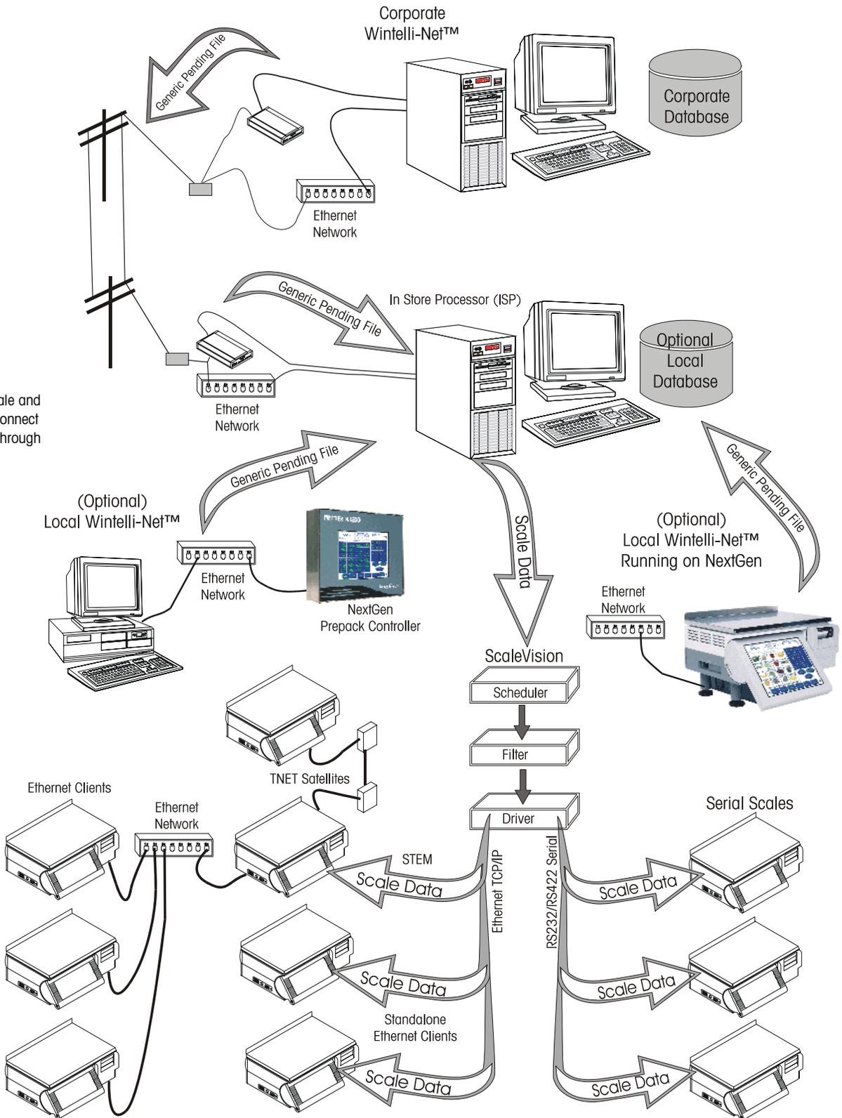
Overview of Wintelli-Net™ using ScaleVision® with both Serial and Ethernet Scale Communication
