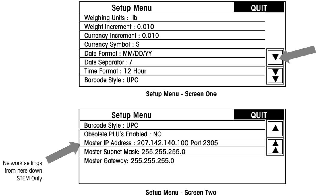
**Figure 3-1: Setup Master Screens, Version 1 STEM**
