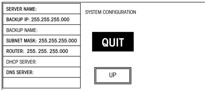
**Figure 3-2: Network Setup Menu Screen Two**
