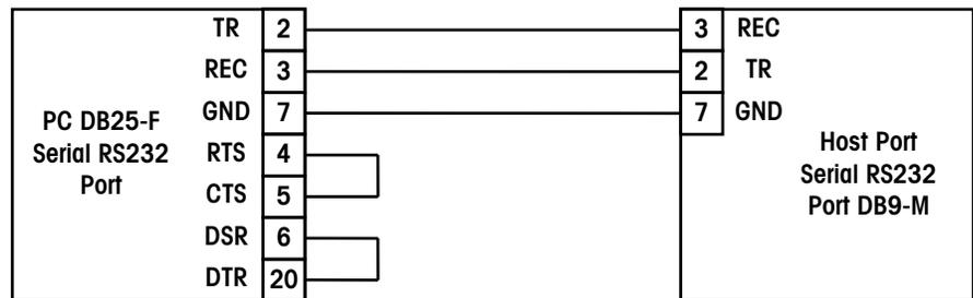
SmartTouch® Master or STEM to PC RS232 Serial Port Wiring
