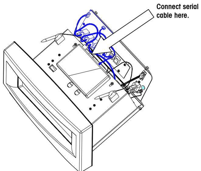
Connecting a Serial Cable to Mercury-PC installed in Model 8361
