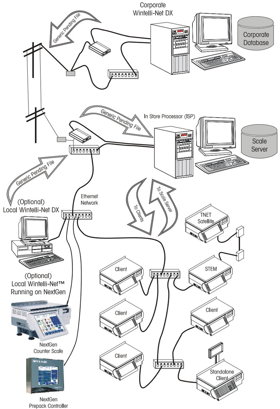
The NextGen Counter Scale and Prepack Controller can connect directly to the database through the Ethernet Network. Scale Server is not needed in this case. The Scale Server is used for proprietary scale data communications.
