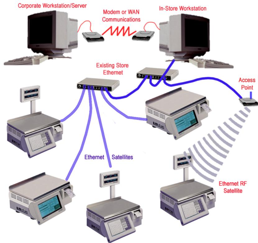
**Ethernet Network with Ethernet RF Scales**
