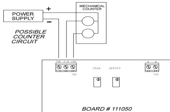
FIGURE 2-6 MECHANICAL COUNTER WIRING
