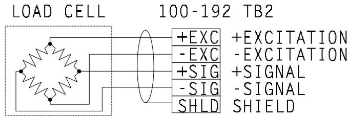
FIGURE 2-2. LOAD CELL TERMINATION
