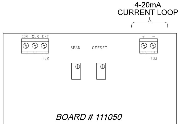
FIGURE 2-4. ANALOG OUTPUT WIRING
