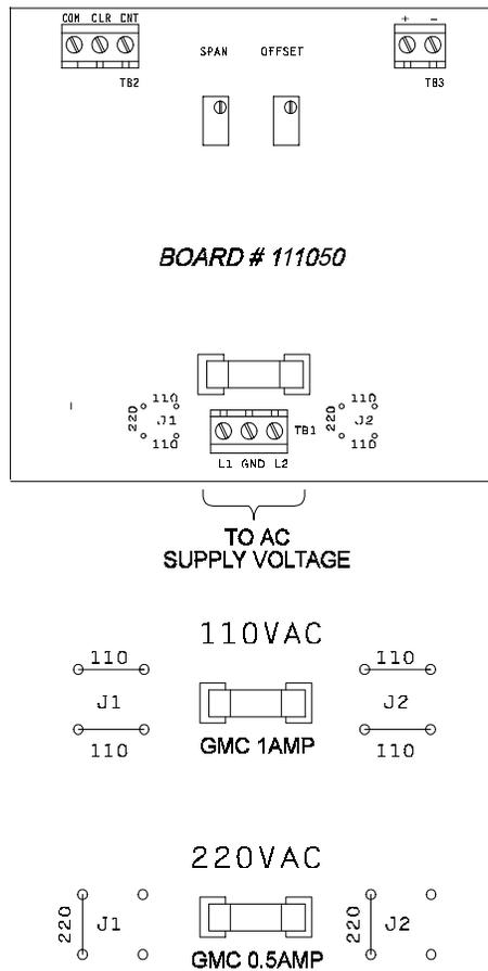
FIGURE 2-1. AC POWER WIRING
