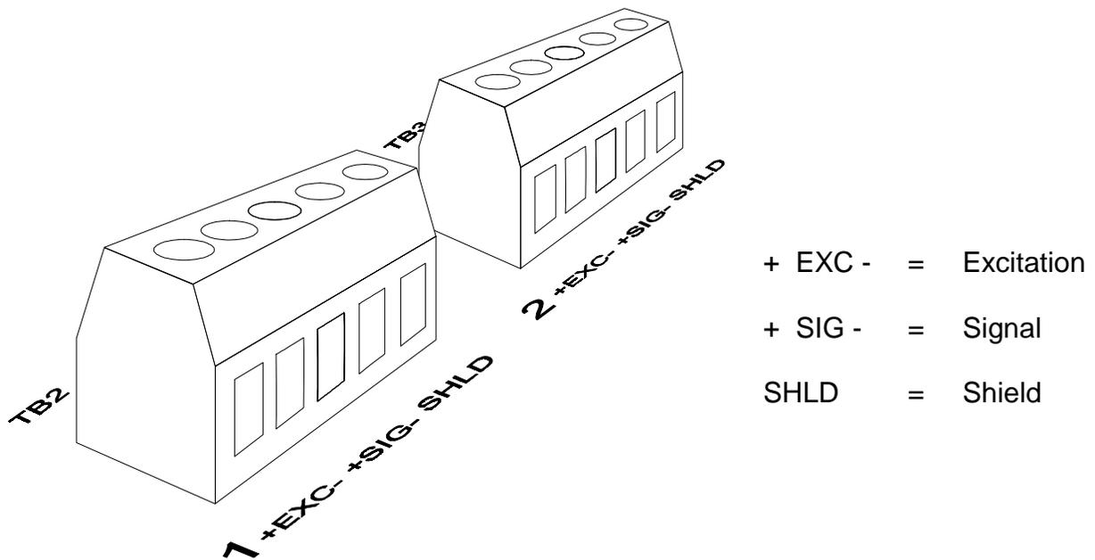
**Figure 3** Load Cell Terminal Blocks
