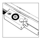
To fasten an antitheft locking device, use the lug (16) located on the rear panel of the balance.
