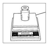
Center the calibration weight on the weighing pan. The balance then calibrates automatically. At the end of calibration, the calibration weight readout and the stability symbol "g" are displayed.
