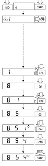
The current code setting in the balance operating menu is identified by a small, superscript "o" after the last number. When you access the operating menu, the previously set code will be displayed after you have selected the right-hand number, which means the entire menu code setting will be displayed. This makes it easy for you to check the previously set menu codes.
