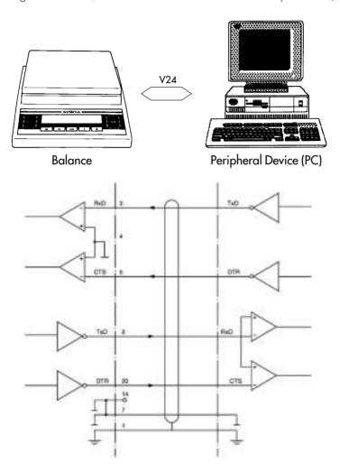
Type of cable: AWG 24 specification
