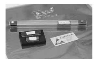
Fold the open end of the bag and seal with tape or a warning label declaring the contents static sensitive. If using clear DIP tubes or conductive foam for IC's, they must also be enclosed in a static shielding bag.
