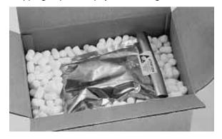
Pink antistatic bubble wrap, foam sheets, foam peanuts, or other antistatic padding may be used to physically protect the component from damage due to rough handling during shipping.
