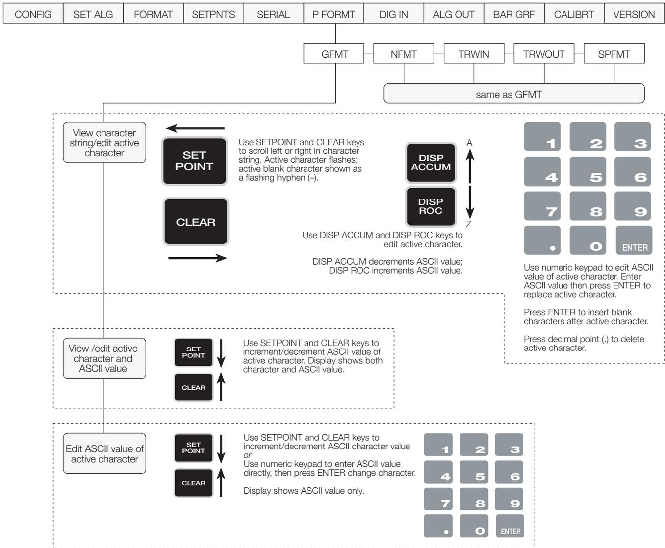
Figure 9. P FORMT Menu, Showing Alphanumeric Character Entry Procedure
