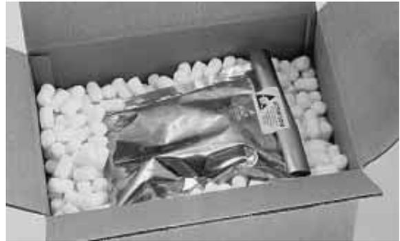
Pink antistatic bubble wrap, foam sheets, foam peanuts, or other antistatic padding may be used to physically protect the component from damage due to rough handling during shipping.
