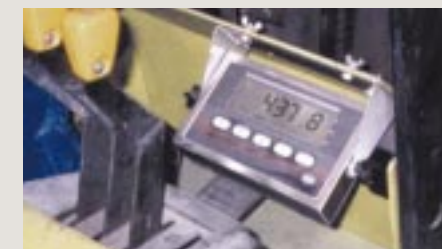
A new battery-operated weight indicator undergoes "real world" testing for dust integrity and shock resistance in a fork-lift application.
