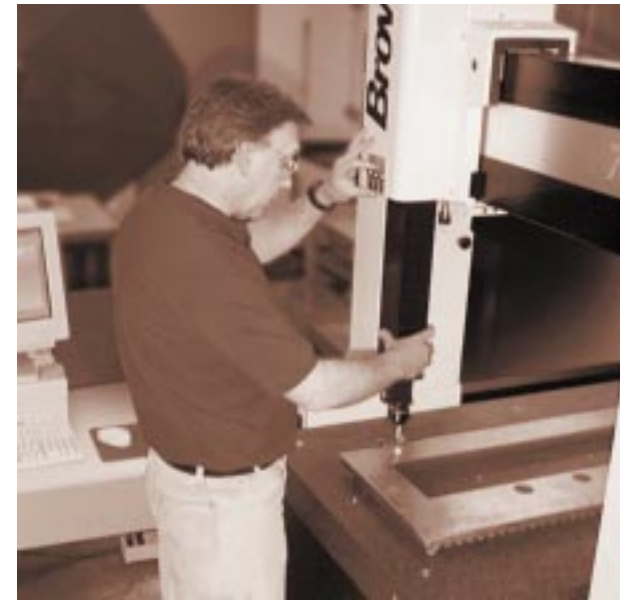
Quality supervisor Dennis Wood uses a coordinate measuring machine on a remote display door sample to ensure proper mounting-hole positions before the finishing process.
