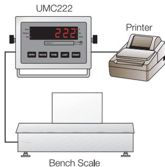
*The UMC222 allows you to calculate and print individual and accumulated weights. It also offers customized ticket formats with time/date and sequential numbering.*
