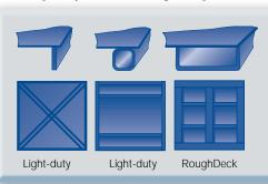
carries a full five-year warranty on the deck structure. The cross sections shown compare the deck structure of the RoughDeck with other low-profile floor scales. The placement of underdeck supports on the RoughDeck minimizes deflection
