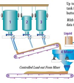
Conveyor motion is activated by the IQ plus 810, as well as mixer activity and timed dispatch of a liquid ingredient into the mixer hopper. Our unique RATTLETRAP® feature filters vibration out of the digital signal, providing accurate, stable weighments.
