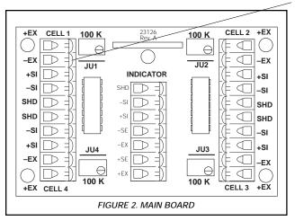
The INDICATOR terminal strip is used to connect the main cable to the indicator. Determine the indicator's load cell input connections from the operating manual. Run a cable from your indicator terminal into the junction box through the larger cord grip and make the connections on the INDICATOR terminal.
