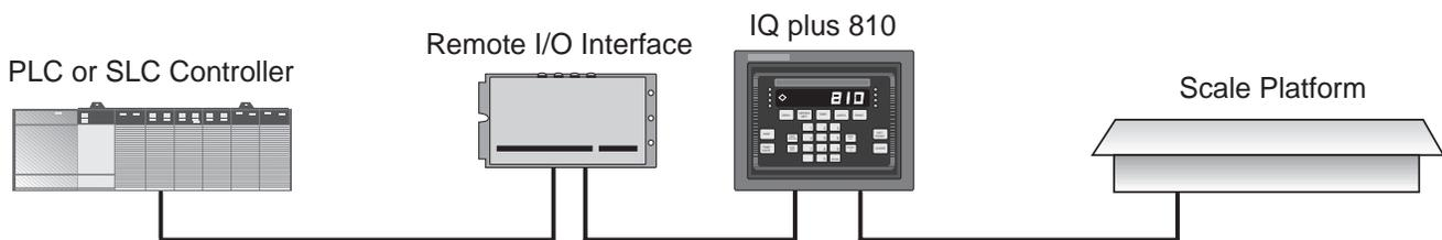
**Figure 8-36. AB Remote I/O Interface Sample Application**
