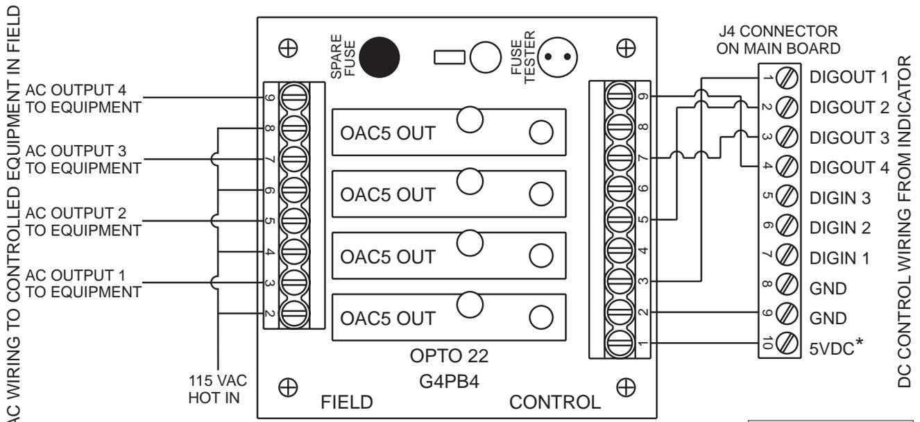
\*NOTE: Boards manufactured prior to August, 1996 may not have 5 VDC power supplied to J4, pin 10. To provide 5 VDC power for digital output operation with those boards, use external power supply board (part # 16418) as shown at right.
