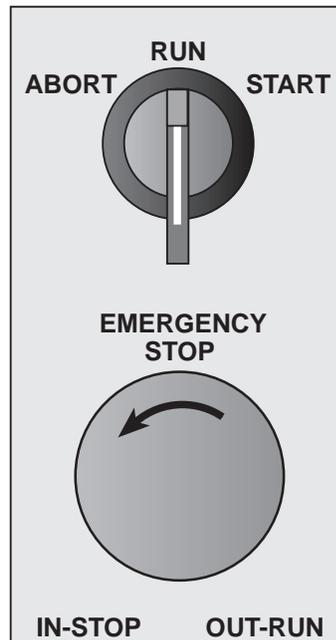
Both switches are wired into the indicator's digital input connection terminal according to the wiring in Figure 8-27 on the following page. Each switch requires a separate digital input, leaving one of the IQ plus 800/810's original three digital inputs available for other use. The 5-VDC digital ground required to operate the switches is available on the indicator's digital input terminal at J4-8 or J4-9.
