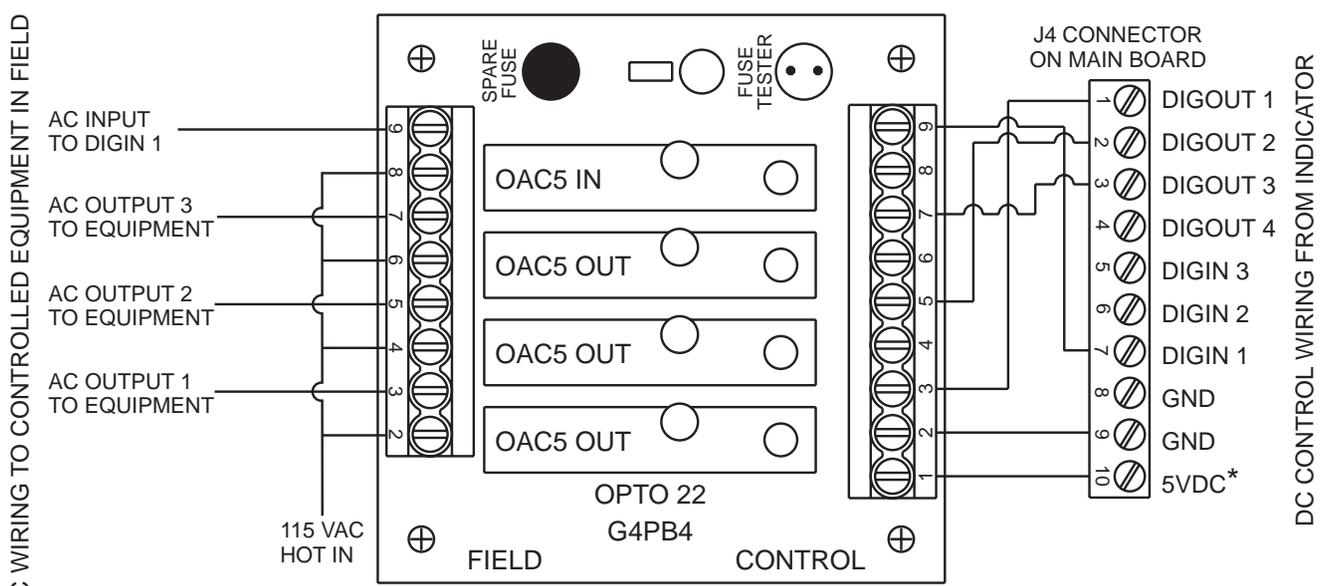
\*NOTE: Boards manufactured after August, 1996 (rev. 2 or higher) have a 5 VDC supply at J4, pin 10 which can be used to power digital outputs on relay boards.
