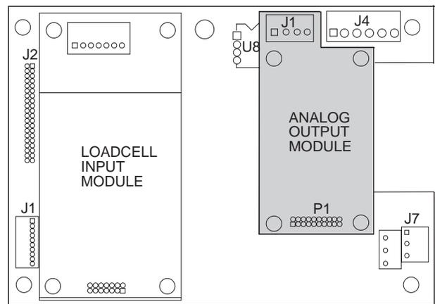
**Figure 8-7. Expansion board with modules installed (component side)**
