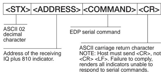
If the initiating address matches the port address of an IQ plus® 800/810 listening on the RS-485 network, that indicator responds.
