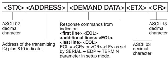
For example, suppose you wish to send the remote print command, KPRINT, from an ASCII terminal to an indicator on the RS-485 network. Assume the indicator’s address is ASCII decimal character 65. After consulting an ASCII chart, you determine that the keyboard equivalent for the STX character (02) is CONTROL-B. The address (65) corresponds to the capital letter “A” and the CR character is ENTER. Therefore, from the terminal you press: CONTROL-B, A, K, P, R, I, N, T, ENTER.
