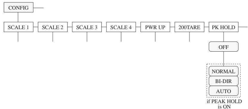
**Figure 8-2. Peak Hold submenu layout**
