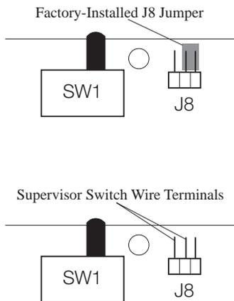
**Figure 8-25. Supervisor Switch Wiring**
