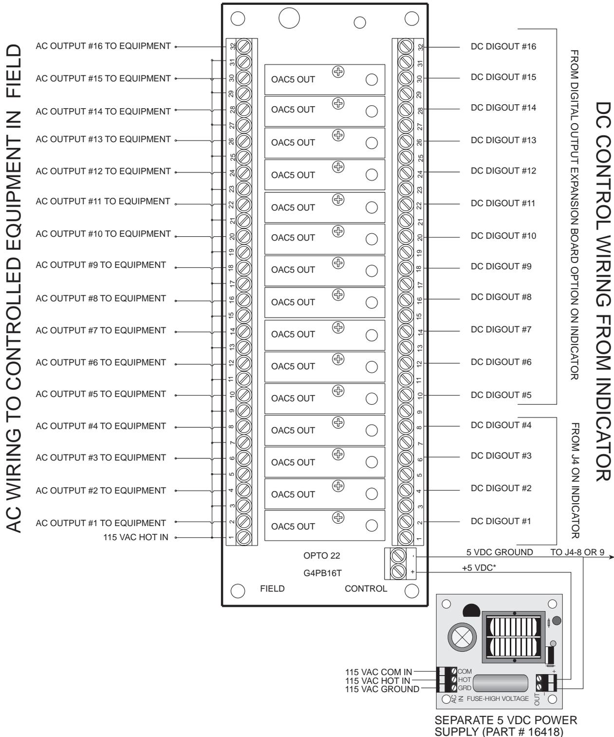
\*When using a main CPU board manufactured after August, 1996 (rev. 2 or higher), +5VDC power can be provided to the relay board from J4-10 on the main board. Boards manufactured prior to that date must use the separate 5 VDC power supply to energize the relay board. In either case, run a 5 VDC ground wire to J4-8 or J4-9.
