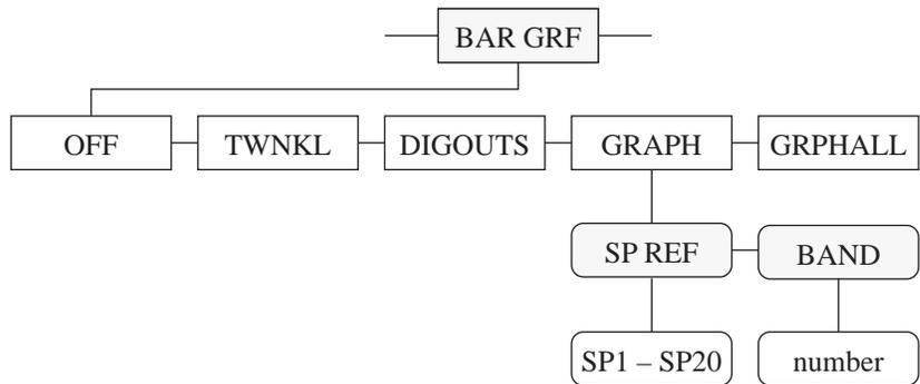
**Figure 8-3. Bar Graph submenu layout**
