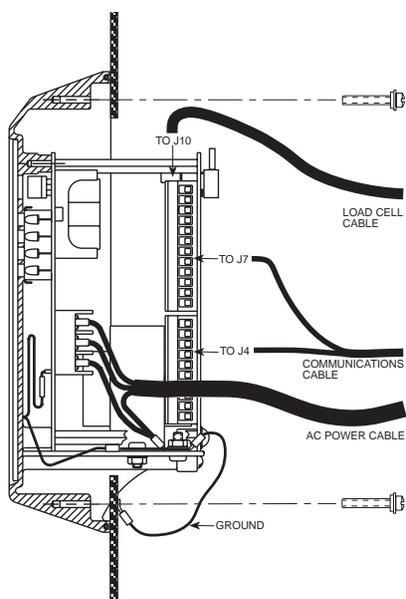
5. Hold the faceplate against the panel as shown and secure with the five machine screws and washers provided.
