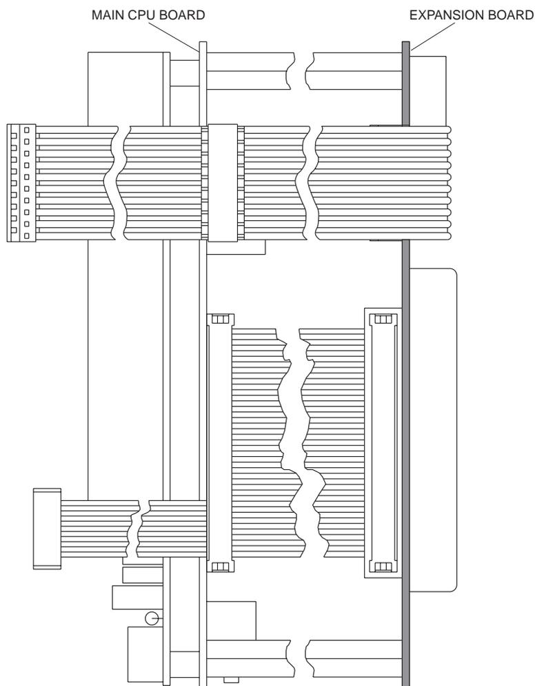
**Figure 8-5. Expansion board (side view)**
