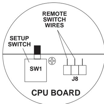
Wiring the remote supervisor switch
