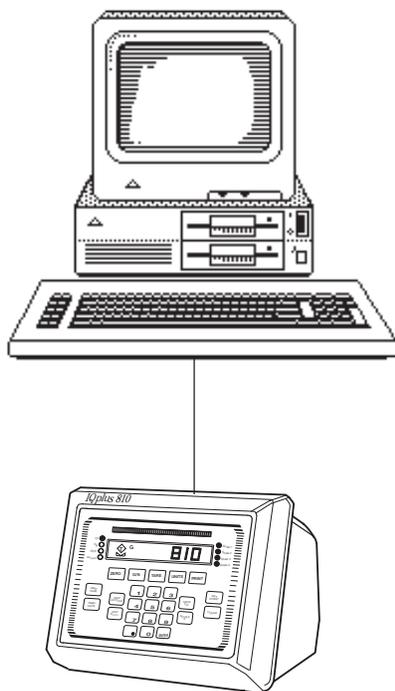
The EDP (electronic data processing) port lets you control the IQ plus 800/810 from a remote keyboard or personal computer. You can transfer configuration data directly between two IQ plus 800/810 indicators. By using special commands from the keyboard, you can simulate front panel key press functions, call up current settings for setup parameters, and perform reporting functions. Also, you can use special commands to transmit weight data directly from the EDP port on demand.
