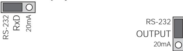
Figure 2-5. *RxD* and *OUTPUT* Jumpers, Showing Jumper Positions for RS-232 Communications
