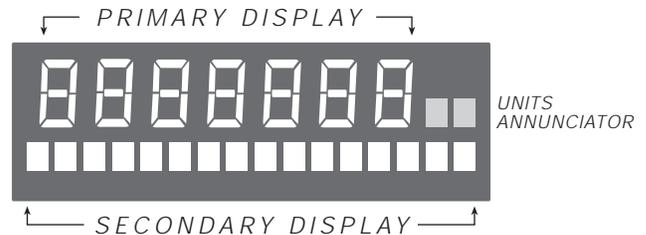
*Figure 1. IQ plus 510 Front Panel Display Areas*
