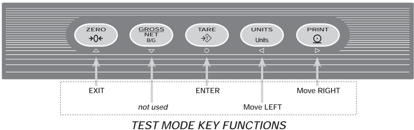
Figure 7-6. Front Panel Key Functions in Test Mode
