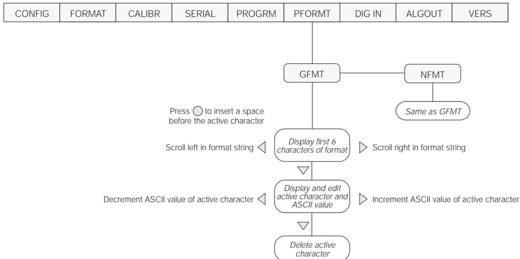
Figure 6-1. PFORMT Menu, Showing Alphanumeric Character Entry Procedure
