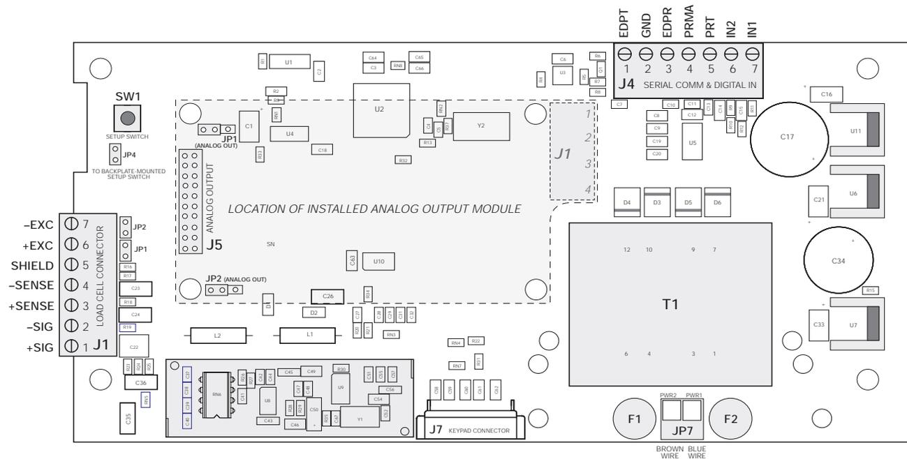
Figure 2-3. IQ plus 350 CPU and Power Supply Board
