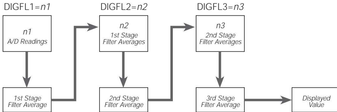
Figure 7-3. Flow Diagram for IQ plus 350 Digital Filters
