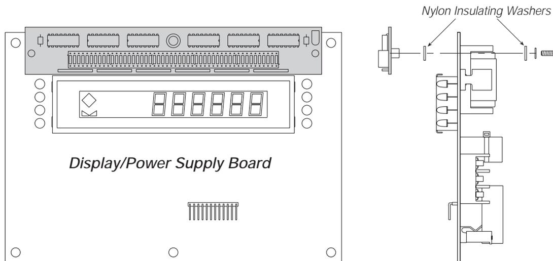
Figure 9-5. Bar Graph Option Installed on Display Board
