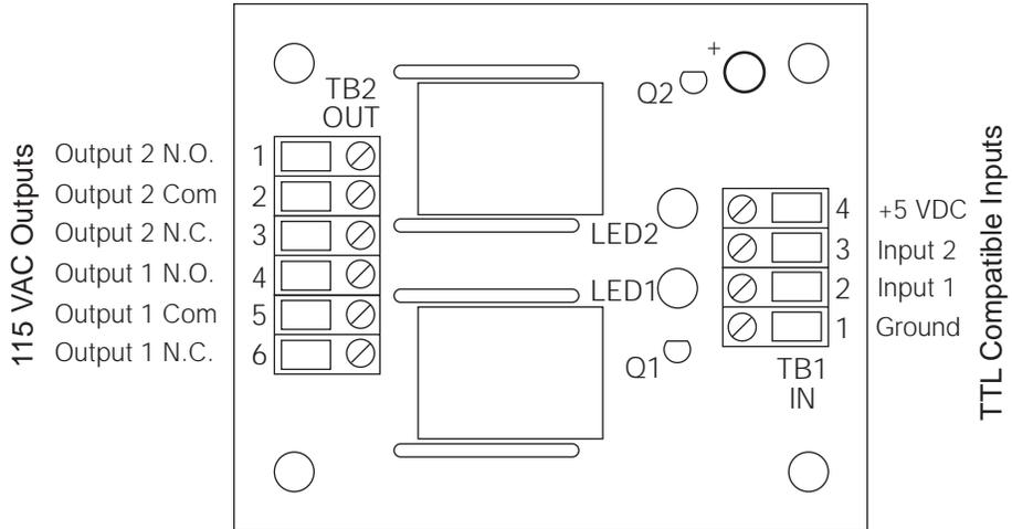
Figure 9-14. IQ plus 800 2-Channel Relay Board, PN 30549
