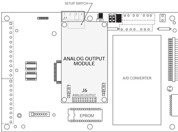
Figure 9-10. Analog Output Installed on CPU Board
