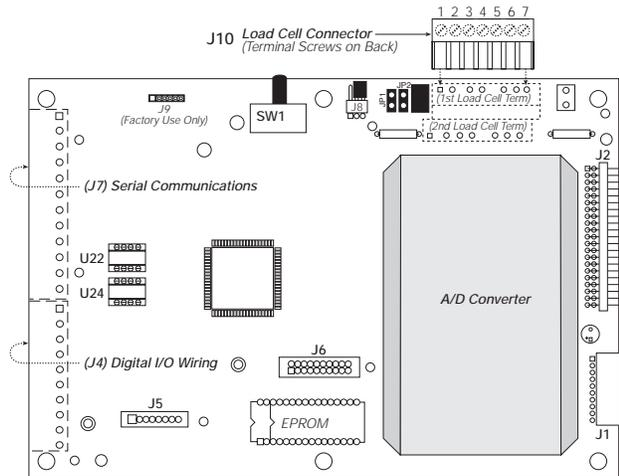
Figure 9-7. Location of Chips U22 and U24 on CPU Board
