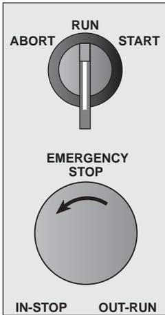
For SS and HE models, the unit can be mounted directly on the face of the case by drilling 7/8" holes for the two switches. Desktop models have insufficient room for switches on the case; a special FRP case is available for mounting the switch unit remotely. The remote mounting kit includes case, 5 feet of cable, O-ring, and cord grip for sealing the cable connection to the indicator. Either mounting method is waterproof and maintains a NEMA 4X rating.
