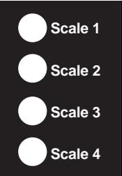
The scale channel LEDs on the right side of the display indicate which scale weight is displayed. See the description of the SCALE # key for more information.
