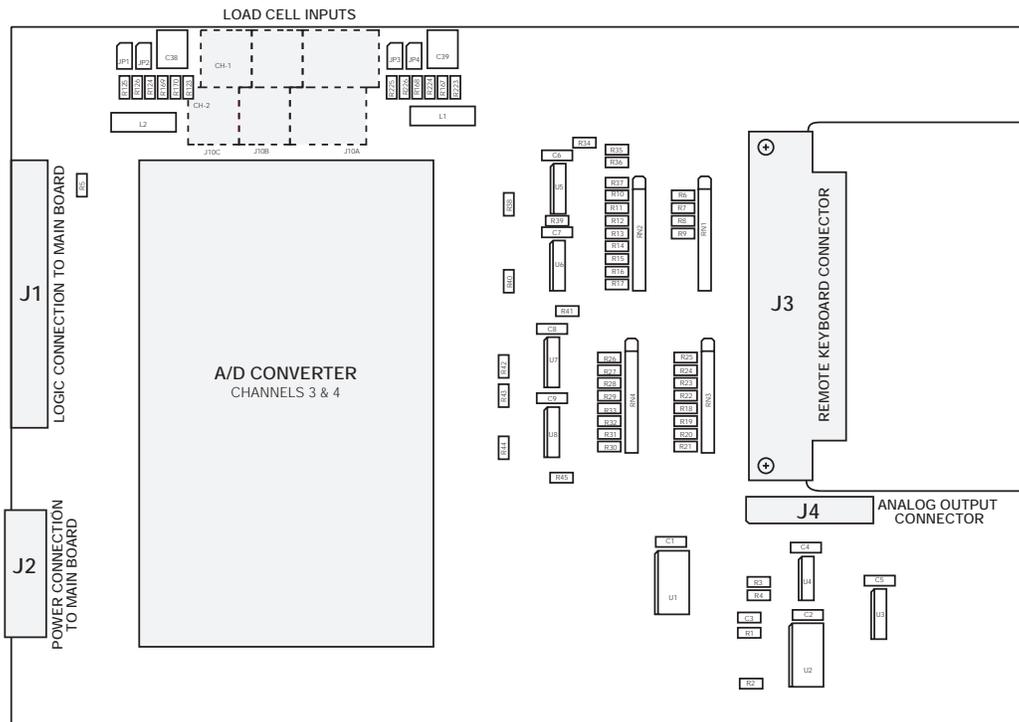
Figure 9-9. IQ plus 810 Expansion Board
