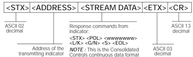
Figure 10-5. RS-485 Continuous Data Format
