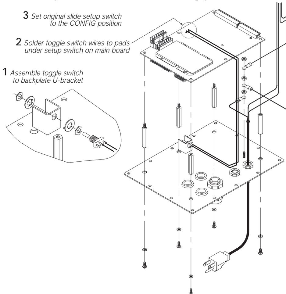
Figure 9-12. IQ plus 800 Replacement Setup Switch Installation
