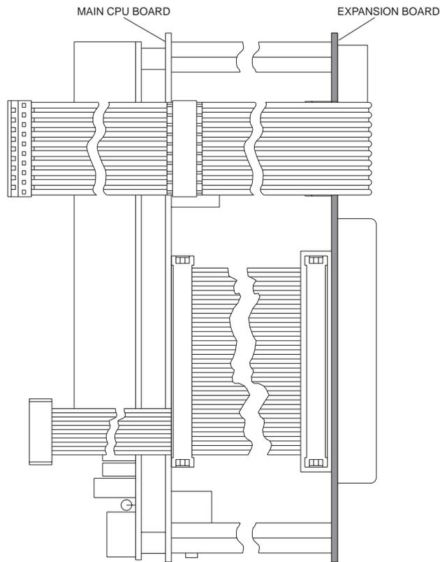
Figure 9-8. Installed Expansion Board, Side View
