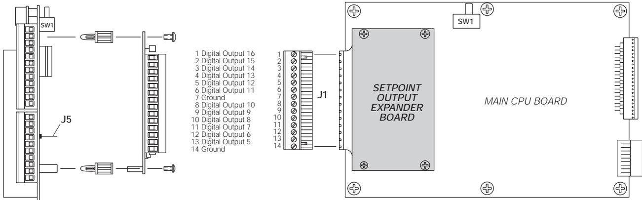
Figure 9-16. Setpoint Digital Output Expansion Board
