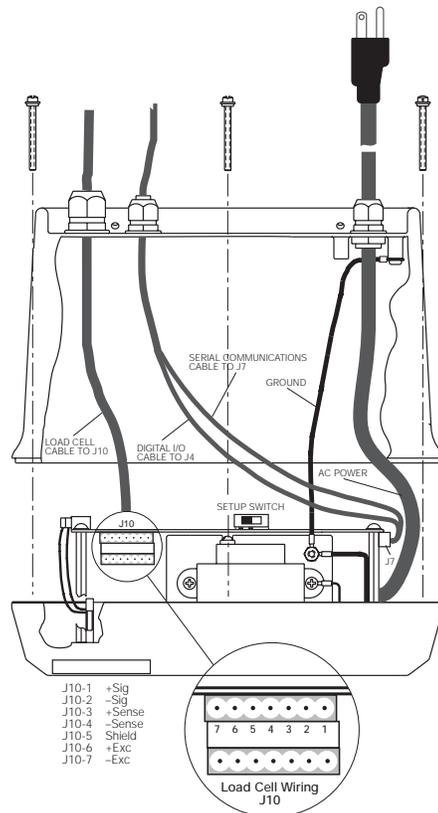
Figure 2-2. IQ plus 810 DT Wiring, Top View
