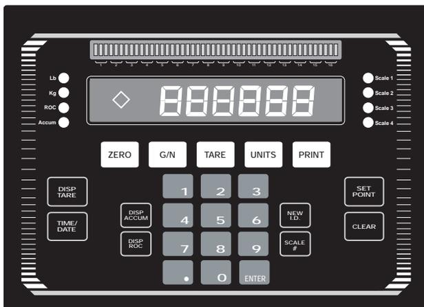
Figure 1-1. IQ plus 810 DT Front Panel
