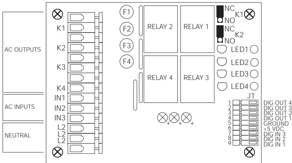
Figure 9-15. IQ plus 800 4-Channel Relay Board, PN 36080
