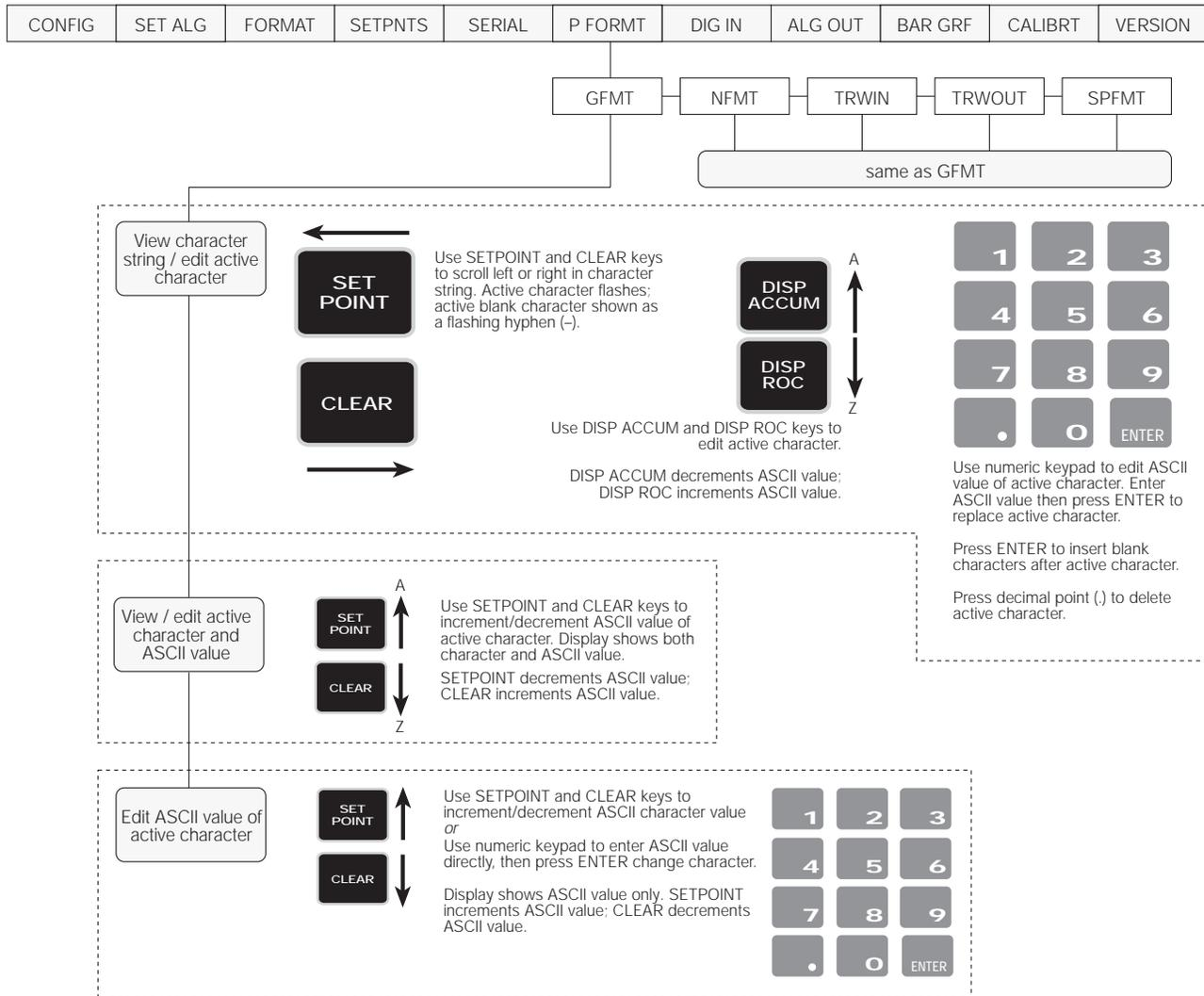
Figure 7-1. P FORMT Menu, Showing Alphanumeric Character Entry Procedure
