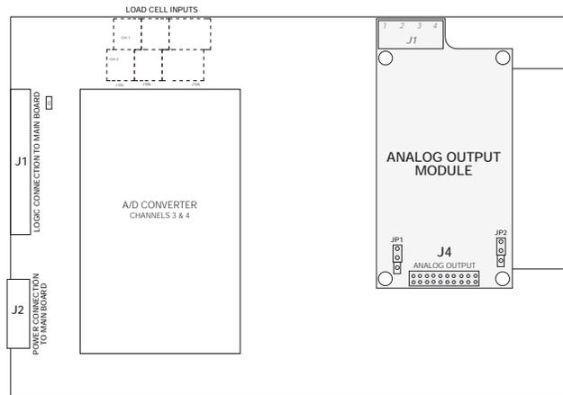
Figure 9-11. Analog Output Installed on Expansion Board
