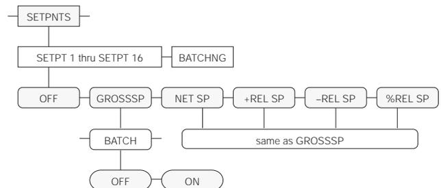
Figure 8-3. Setpoint BATCH Parameter
