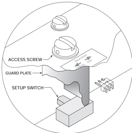
Figure 3-1. IQ plus 800 Setup Switch Access
