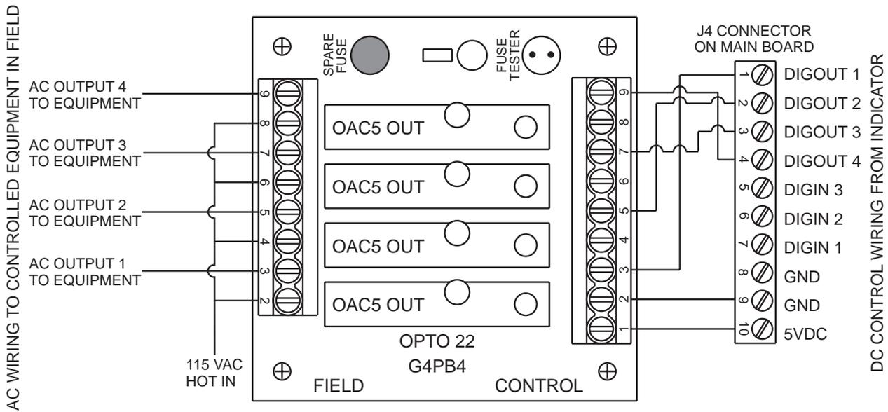
Figure 9-19. Relay Wiring for 4 AC Outputs
