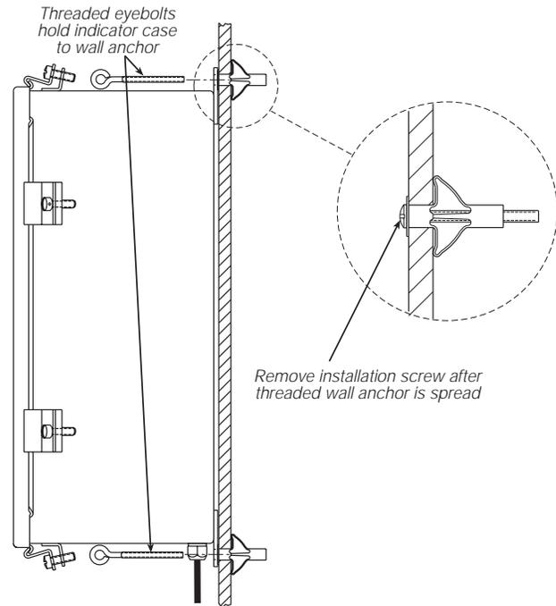
Figure 2-12. Wall Mounting for HE and SS Models
