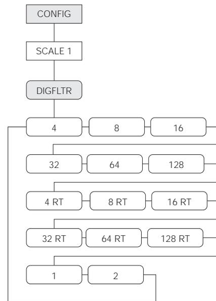
Figure 10-6. Digital Filtering Submenu
