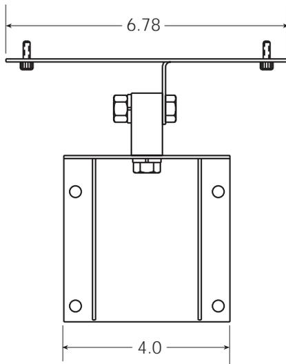
Figure 2-11. IQ plus 810 DT Wall Mount (Front View)
