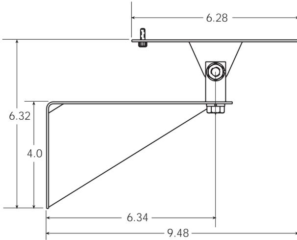
Figure 2-10. IQ plus 810 DT Wall Mount (Side View)
