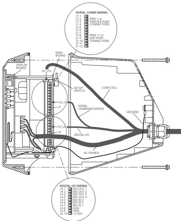
Figure 2-1. IQ plus 810 DT Wiring, Side View
