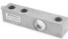
This welded seal precision load cell offers exceptional performance and reliability in hostile environment applications typical of food and chemical processing. Designed for single- or multiple-cell installations, the 65083S is provided with a threaded load hole for easy adaptation of mounting hardware or leveling feet typical of floor scales. Capacities from 1000 to 10,000 lb (453.6 to 4535.9 kg). Integral 20' (6.1m) cable.
