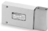
Load cells especially designed for heavy-duty, off-center loads on a 20" x 20" (508mm x 508mm) platform. Stainless steel construction specially designed for washdown situations. Includes integral 10' (3.1m) cable. 1000 lb (453.6 kg) capacity load cell may be used with 30" x 30" (762mm x 762mm) platform. Capacities from 25 to 1000 lb (11.3 to 453.6 kg).
