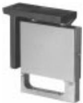
Low-capacity load cell designed for single-cell platforms in protected environments. Built-in overload stops protect against overload (up to 5 times rated capacity). Integral 10' (3.1m) cable. 1 to 10 lb (.5 to 4.5 kg) cells may be used with a base size of 6" x 6" (152.4mm x 152.4mm); 20 to 100 lb (9.1 to 45.4 kg) cells, with a base size of 12" x 12" (304.8mm x 304.8mm).
