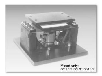
The MagnaMount tank, truck and railroad scale assembly is designed for use with Rice Lake Weighing Systems' RLCSP1 or Revere Transducer's CP1 or CSP1 load cells. The "Shielded Cell" load cell mounting assembly is a highly reliable design that shields the load cell from shock and side load effects, assuring accurate weighing even under adverse loading conditions.
