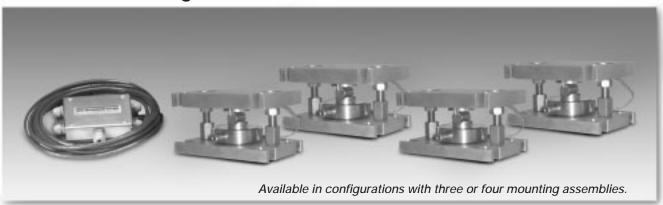
The 220 Universal Mount is designed to be used with the Model 220 load cell described above. The mount incorporates built-in jacking bolts to prevent damage to the load cell during installation. It's stainless steel construction is designed to be used in the harshest of environments.
