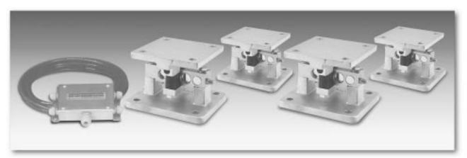
Incorporating an articulating load plate, hardened load pin and double-ended beam load cell into one simple design, the 2100HE tolerates eccentric loads and side loads of up to 100% of capacity.
