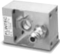
This high-accuracy stainless steel single-point load cell is an ideal replacement cell for hopper applications where damaged bellows are a problem. This cell also features complete hermetic sealing, making it suitable for use in the toughest environments. This product is offered at 150 lb (68.0 kg), and comes complete with 10' (3.1m) of load cell cable.
