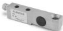
The SB5 stainless steel single-ended beam is designed for multiple-cell applications such as floor scales and tank, bin and hopper weighing systems. It is used exclusively in Rice Lake Weighing Systems' Paramounts® EP mounting systems. Millivolt/volt/ohm factory calibration assures matched outputs for easy calibration. NTEP-certified capacities from 1125 to 11,250 lb (5 kN to 50 kN/510.3 to 5102.9 kg); Non-NTEP capacity of 22,500 lb (100 kN/ 10,2025.8 kg).
