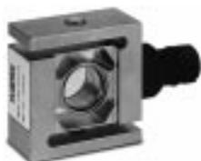
The UB6 stainless steel S-beam is designed to meet the most stringent accuracy requirements. Exclusive 10' (3.1m) field-replaceable load cell cable simplifies cable and load cell repairs. Capacities from 225 to 1125 lb (1kN to 5kN/102.1 to 510.3 kg).
