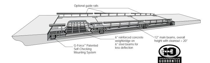
Package includes: Assembled weighbridge modules and weighbridge fasteners; load cells with conduit fitting; load cell mounts with leveling bolts and anchor bolts; copper transient bypass cables at each load cell; metal conduit on weighbridge for load cell cable runs; flexible plastic conduit from load cell to metal conduit; conduit fittings from plastic to metal conduit; FRP junction box(es); homerun cable to indicator (60' long); print packages including foundation drawing (pier or
